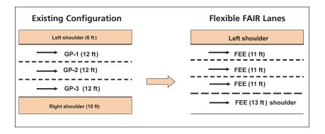
FIGURE 4 Conversion of six-lane highway to FEE highway.
