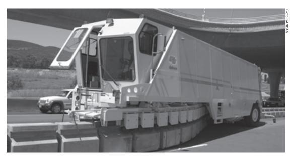
A barrier transfer machine moves Jersey barriers to reallocate a traffic lane on I-15. The reversible lane segment of I-15 will be widened as part of the facility's expansion.
