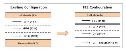
FIGURE 1 Creating flexible lanes on a six-lane highway.
