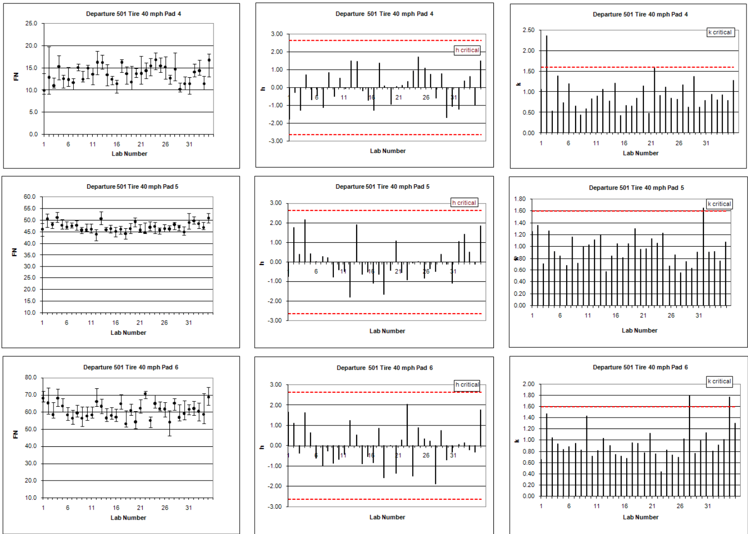
Figure 2-9- Box plots and h and k statistics for friction numbers of TRC Departure State System with 501 tire at 40 mph
