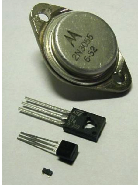
FIGURE 1-2 Assorted discrete transistors from Motorola and Siemens Technologies. SOURCE: Courtesy of Wikipedia. Used with permission from Daniel Ryde.
