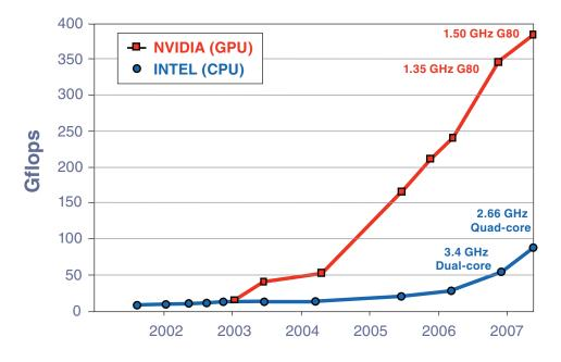
FIGURE 2-5 GPUs, a core technology for games, are greatly outpacing commodity CPUs. SOURCE: Dunning (2009).
