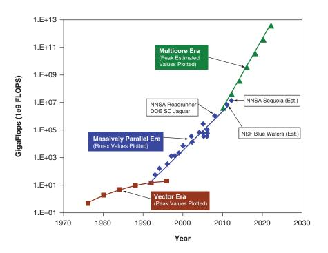
FIGURE 2-2 Rapid growth in computing capability spanning eras of vector, massively parallel, and future multicore trends. SOURCE: Vector era and massively parallel era data from Top 500 (http://www.top500.org/); multicore era data notional based on aggressive growth.
