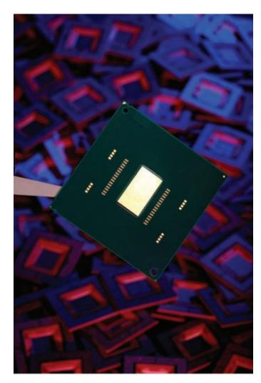
FIGURE 2-3 Intel's 1 teraflop on a chip (275 mm<sup>2</sup> and 62-watt power consumption), demonstrated in 2007. This single chip contains 80 cores, hence the term "multicore." SOURCE: See http://techresearch.intel.com/articles/ Tera-Scale/1449.htm. Accessed May 27, 2009. Reprinted with permission of Intel Corporation.
