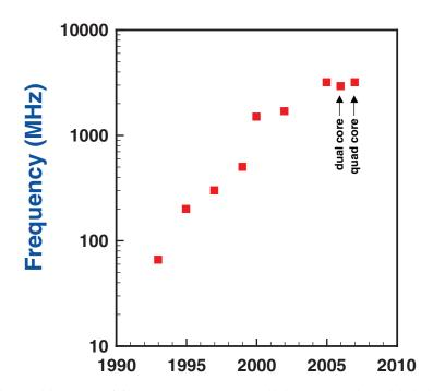
FIGURE 2-4 Clock speed in terms of frequency versus year. All data except those labeled refer to single-core processors. Even with additional cores added to a chip, the chip clock speed has currently reached an asymptote. SOURCE: Dunning (2009).
