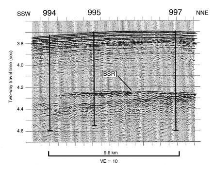
**FIGURE 2.5** Seismic reflection profile (CH-06-92 Line 31) across the Blake Ridge along which the Ocean Drilling Program Leg 164 drilled a three-hole transect to identify the origins of the BSR. SOURCE: Charles Paull.
