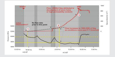
Cumulative production (red line) and derived bottom-hole pressure (black line) from pressure drawdown test at Mallik. Operational issues during which the pump did not operate are shown with dark gray vertical shading. A peak flow of more than 5,000 m<sup>3</sup>/day was achieved near the end of the test. SOURCE: After Dallimore et al. (2008).
