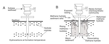
**FIGURE 2.7** Potential changes at the wellhead induced by methane venting: (A) initial conditions and (B) the changes induced by methane venting outside the casing. SOURCE: Borowski and Paull (1997).
