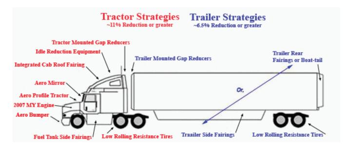
**FIGURE 3-7** Some of the aerodynamic technologies included in the SmartWay certification program. SOURCE: Mitch Greenberg, EPA, "SmartWay Voluntary Certification Program," presentation to the committee.
