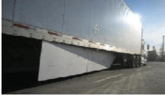
FIGURE 5-11 ATDynamics trailer tail (left) and FreightWing trailer skirt (right). SOURCE: Courtesy of Freight Wing.
