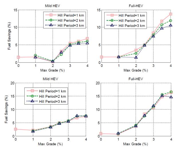
**FIGURE 4-24** Fuel savings of hybrid trucks with respect to conventional trucks as a function of maximum grade for various hill periods; (left) 50 percent load and (right) 100 percent load. SOURCE: ANL (2009).
