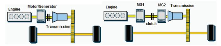
FIGURE 4-17 Hybrid configurations considered in ANL study. SOURCE: ANL (2009).
