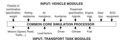
FIGURE 3-1 Overview of simulation tool and methodology proposed for use in the European Union. Both inputs and results are declared transparently. SOURCE: Stefan Larsson, European Auto Manufacturers, presentation to the committee.
