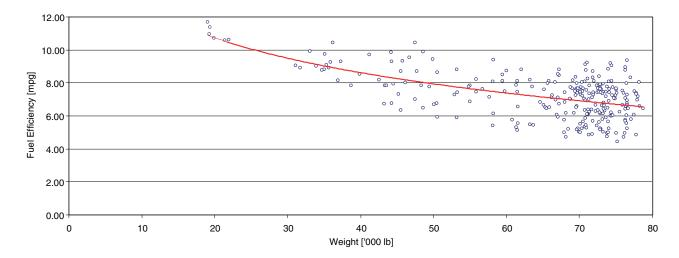
**FIGURE 5-37.** Effect of weight on truck fuel economy for a monitored fleet of six trucks with combination of dual and wide single tires for a variety of drive routes. SOURCE: Capps et al. (2008).
