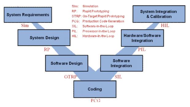
FIGURE H-1 V diagram for software development.
