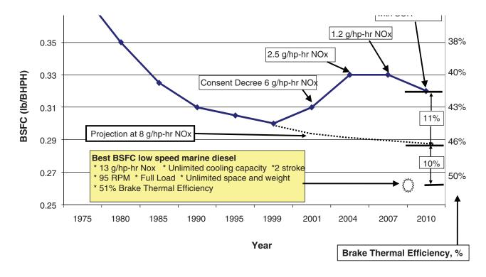
**FIGURE 4-2** Historical trend of heavy-duty truck engine fuel consumption as a function of  $NO_x$  requirement. SOURCE: Tony Greszler, Volvo, October 2009.
