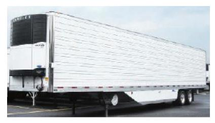
FIGURE 5-18 Refrigerated van trailer with Freight Wing skirts. SOURCE: Courtesy of Freight Wing.
