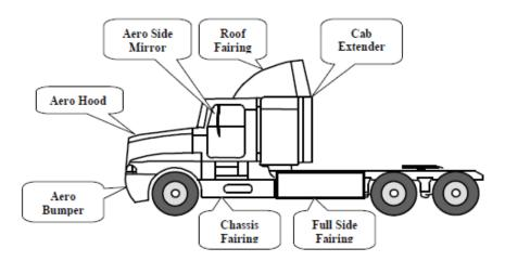
FIGURE 5-5 Aerodynamic sleeper tractor aerodynamic feature identification.
