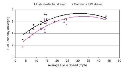
**FIGURE 2-15** Curves based on chassis dynamometer for fuel economy versus average speed for conventional and hybrid buses. SOURCE: Wayne et al. (2008). Reprinted with permission from the Transportation Research Forum.
