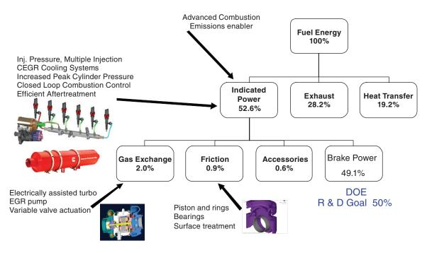
**FIGURE 4-3** Research roadmap for 49.1 percent thermal efficiency by 2016. SOURCE: Provided under license by Cummins Inc. Copyright 2009 Cummins Inc. All rights reserved.
