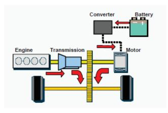
**FIGURE 4-12** Example of post-transmission configuration. Courtesy of University of Michigan.
