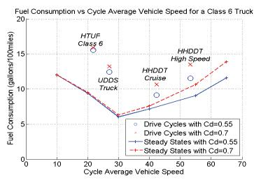
**FIGURE 2-12** PSAT simulation results for steady-state operation and for selected transient test cycles for a Class 8 truck (top) and a Class 6 truck (bottom). The Class 6 truck modeled at 9,070 kg was based on a GMC C Series, and the Class 8 truck modeled at 29,931 kg was based on a Kenworth T660 with Cummins 14.9 L ISX. SOURCE: ANL (2009), Figures 26 and 28.
