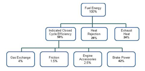
FIGURE 4-1 Energy audit for a typical diesel engine.
