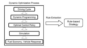
**FIGURE 4-25** Dynamic programming process and rule extraction from the result. SOURCE: Lin et al. (2003).
