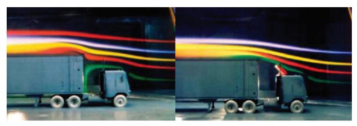
**FIGURE 5-3** National Research Council of Canada: Smoke pictures, cab with deflector (right). SOURCE: Cooper (2004), p. 11, Fig. 2. Reprinted with kind permission of Springer Science and Business Media.
