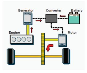
**FIGURE 4-7** Series hybrid electric vehicle. Courtesy of University of Michigan.
