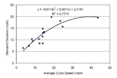
**FIGURE 2-13** Standard deviation of speed changes (coefficient of variance rises) as the average speed drops for typical bus activity. SOURCE: Wayne et al. (2008). Reprinted with permission from the Transportation Research Forum.
