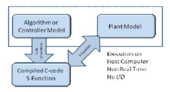
FIGURE H-7 Software-in-the-loop.
