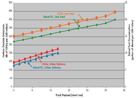
FIGURE 2-5 Fuel consumption versus payload SOURCE: Jeffrey Seger, Cummins, Inc., personal communication, June 6, 2009.
