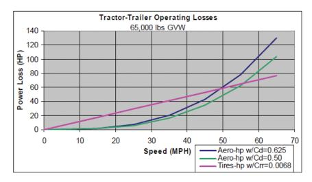
FIGURE 5-7 Aerodynamic and tire power losses for tractor-van trailer combination.
