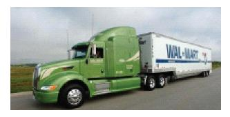
**FIGURE 5-24** Walmart's 2008 low fuel consumption tractor trailer. SOURCE: Courtesy of Walmart.
