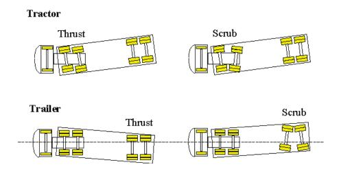
FIGURE 5-31 Tractor-trailer tandem-axle misalignment conditions. SOURCE: Kreeb and Brady (2006).
