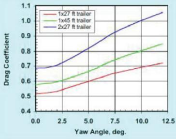
**FIGURE 5-16** Drag coefficient for aerodynamic tractor with single or double trailers. SOURCE: Cooper (2004), p. 17. Reprinted with kind permission of Springer Science and Business Media.
