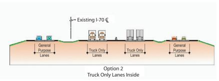
FIGURE 7-3 Example of truck-only lanes. SOURCE: FHWA (2005).
