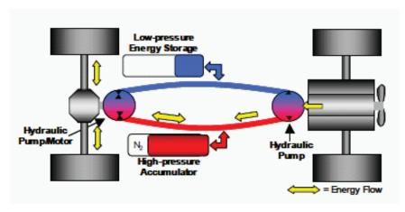
FIGURE 4-8 Series engine hybrid hydraulic vehicle. SOURCE: Eaton-HTUF (2009). Courtesy of Eaton.
