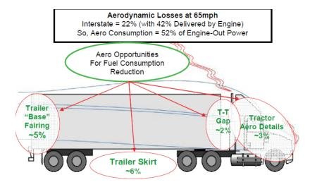
**FIGURE 5-8** Tractor-trailer combination truck showing aerodynamic losses and areas of energy-saving opportunities. Percent changes refer to fuel consumption. SOURCE: Based on Wood (2006). Courtesy of Richard Wood.
