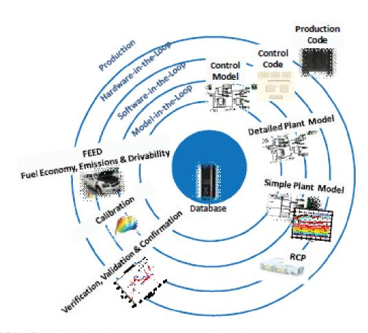
FIGURE H-2 Different levels of modeling required throughout the model-based design process.
