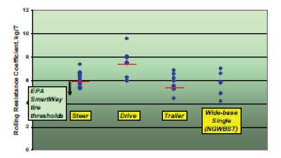
**FIGURE 5-30** Example rolling resistance coefficients for heavy-duty truck tires. SOURCE: Presentation to the committee by C. Bradley and S. Nelson, Michelin Tire North America, "Truck Tires and Rolling Resistance," February 4, 2009. Courtesy of Michelin Tire North America.
