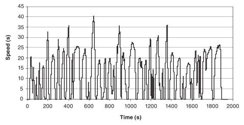
FIGURE 2-11 Orange County Transit Authority cycle derived from transit bus activity data. SOURCE: SAE.
