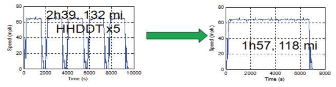
FIGURE 4-21 HHDDT 65 cycle repeated five times with stops (left) and without stops (right). SOURCE: ANL (2009).
