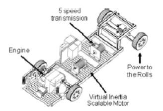
**FIGURE H-12** Several components in the loop—MATT example. SOURCE: Argonne National Laboratory.
