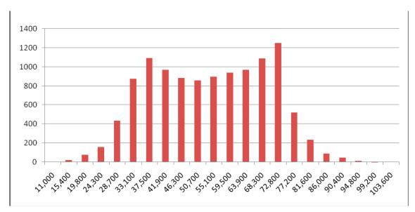
FIGURE 5-35 Truck weight distribution from 2008 weigh-in-motion. SOURCE: New West Technologies.
