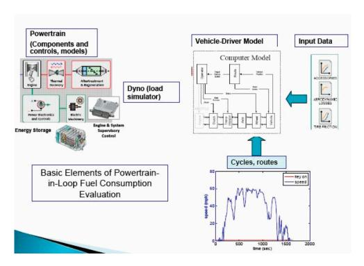
FIGURE 8-4 CIL test of a hybrid vehicle power train to determine vehicle fuel consumption on a specific test route.
