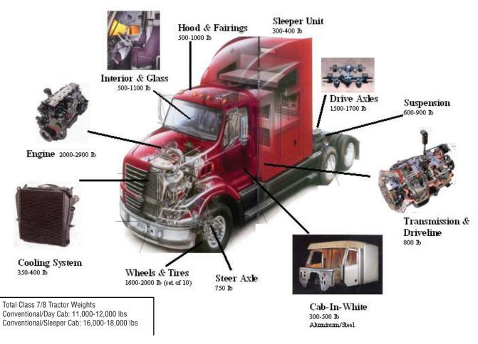
FIGURE 5-33 Typical weights of specific components in Class 8 sleeper tractors. SOURCE: Smith and Eberle (2003).
