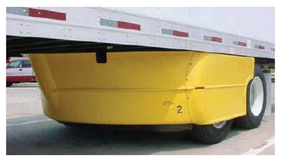
FIGURE 5-14 Trailer bogie cover. SOURCE: TMA (2007).
