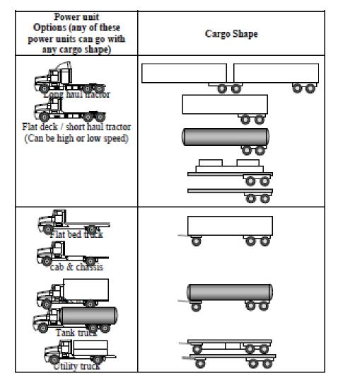
FIGURE 8-2 Illustration of diversity of trailer and power unit (tractor) options.
