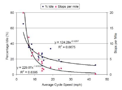
**FIGURE 2-14** Percentage of time spent idling rises and there are more stops per unit distance as the average speed drops for typical bus activity. SOURCE: Wayne et al. (2008). Reprinted with permission from the Transportation Research Forum.
