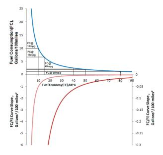
**FIGURE E-1** Fuel consumption (FC) versus fuel economy (FE) (upper half of figure) and slope of FC/FE curve (lower half of figure). The light-colored lower curve matches the left-hand y-axis, while the dark curve matches the right-hand y-axis.
