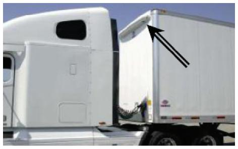
**FIGURE 5-12** Nose cone trailer "eyebrow." SOURCE: Photo provided with permission by FitzGerald Corporation, national marketer for Nose Cone Mfg. Co. Nose Cone is a registered trademark.
