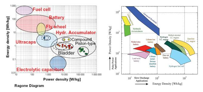
**FIGURE 4-6** Power density versus energy density of various technologies. SOURCE: Baseley et al. (2007). Reprinted with permission from SAE Paper 2007-10-4150. © 2007 SAE International.
