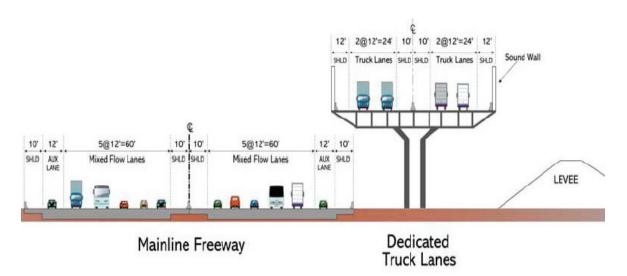
FIGURE 7-5 Elevated truck lanes. SOURCE: FHWA (2005).
