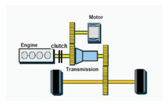
**FIGURE 4-11** Example of pre-transmission parallel configuration. Courtesy of University of Michigan.
