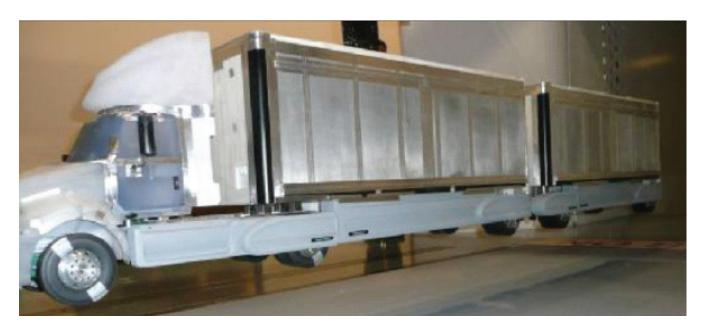
**FIGURE 5-17** Laydon double trailer arrangement with trailer skirts and vortex stabilizers on both trailers; SOURCE: Courtesy of Laydon Composites.
