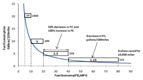
**FIGURE 2-2** Fuel consumption (FC) versus fuel economy (FE), showing the effect of a 50 percent decrease in FC and a 100 percent increase in FE for various values of FE, including fuel saved over 10,000 miles. Results are based on Eq 2-1.
