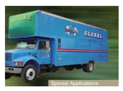
**FIGURE 5-26** Nose Cone fairing on face of straight truck. SOURCE: Photo provided with permission by FitzGerald Corporation, national marketer for Nose Cone Mfg. Co. Nose Cone is a registered trademark.
