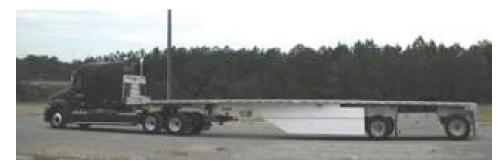
FIGURE 5-19 Freight Wing skirts on flatbed trailer. SOURCE: Courtesy of Freight Wing.
