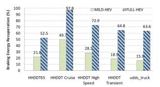
FIGURE 4-19 Percentage of braking energy recovered at the wheels under (left) a 50 percent load and (right) a 100 percent load. SOURCE: ANL (2009).
