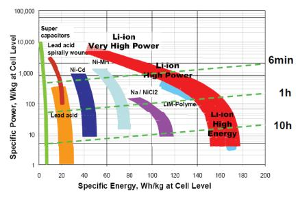
FIGURE 4-15 Battery type versus specific power and energy. SOURCE: Kalhammer et al. (2007).
