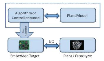
FIGURE H-5 On-target rapid prototyping.
