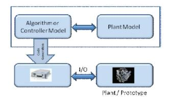
FIGURE H-4 Rapid control prototyping
