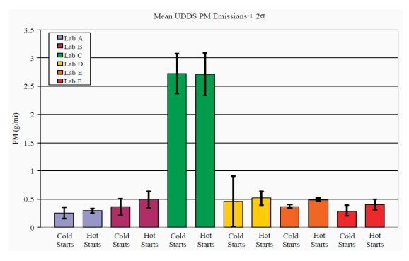
FIGURE H-15 Mean particulate matter results with two standard deviation error bars. SOURCE: Argonne National Laboratory.
