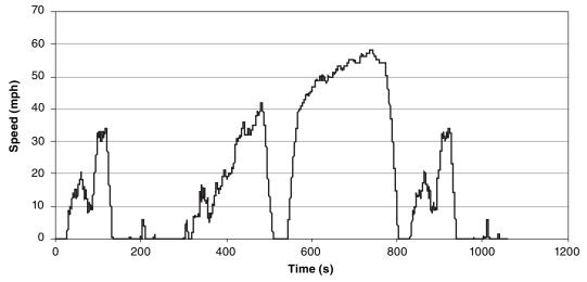
**FIGURE 2-8** The Heavy-Duty Urban Dynamometer Driving Schedule. SOURCE: Clark (2003). Reprinted with permission from SAE. © 2003 SAE International.
