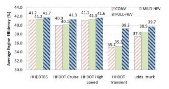
FIGURE 4-20 Percentage average engine efficiency of conventional and hybrid trucks for (left) a 50 percent load and (right) a 100 percent load on standard cycles. SOURCE: ANL (2009).
