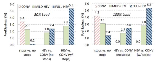
**FIGURE 4-22** Fuel consumption reduction due to stop removal, with respect to conventional vehicles without stops, and with respect to conventional vehicles with stops (50 percent load on the left, 100 percent load on the right). SOURCE: ANL (2009).
