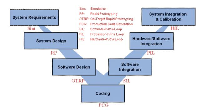
FIGURE 2-16 "V" diagram for software development.
