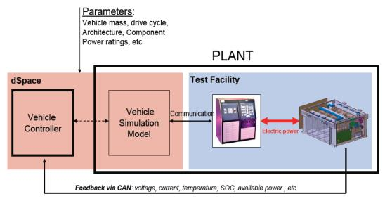
FIGURE H-11 Battery connected to a DC power source. SOURCE: Argonne National Laboratory.
