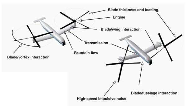
FIGURE 5-2 Breakdown of typical noise sources for a rotorcraft configuration. Source: Burley (2008).
