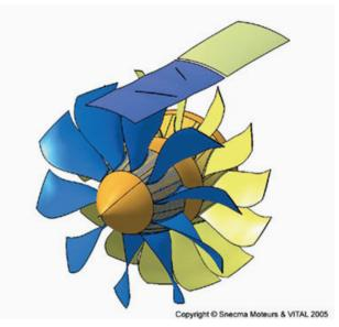
FIGURE 5-14 Schematic drawing of contrarotating turbo fan design to be studied in VITAL. Source: EU (2007).
