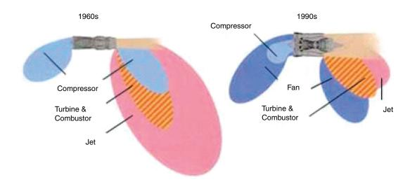
FIGURE 5-3 Noise sources for 1960s and 1990s jet engines. Source: Rolls-Royce (2005a).
