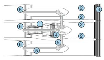
FIGURE 5-13 SAX-40 engine design. Source: SBAC (2009). Copyright Silent Aircraft Initiative.
