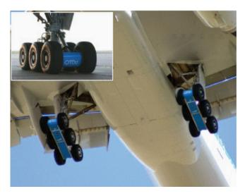
FIGURE 5-5 Toboggan landing gear fairings for reducing landing gear noise tested in QTD2. Source: Herkes (2006). Copyright Boeing. All rights reserved.
