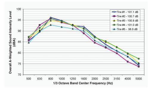
FIGURE 5-19 Range in one-third octave band sound intensity levels for tires measured at 97 kilometers per hour on a dense, graded, asphaltconcrete roadway. Source: Adapted from Donavan (2006).
