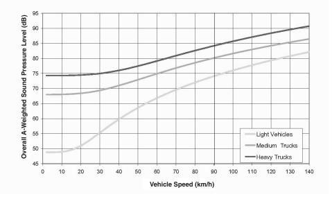
FIGURE 5-16 U.S. average pass-by noise levels under cruise conditions for light vehicles, medium trucks, and heavy trucks measured at a distance of 15 meters. Source: Fleming et al. (1996).
