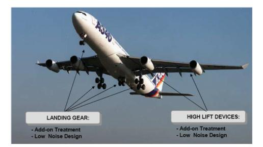
FIGURE 5-10 Aircraft noise reduction technologies. Source: SBAC (2009).
