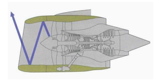
FIGURE 5-11 Negatively scarfed intake reflects fan noise away from the ground. Source: *The Jet Engine*, 2005. Reprinted with permission from Rolls Royce, 2005.
