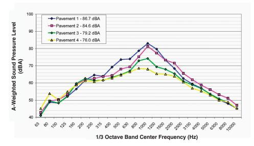
FIGURE 5-20 One-third octave band pass-by noise levels for the same car and tires operating on different pavements at 97 kilometers per hour. Source: Adapted from Donavan (2006).
