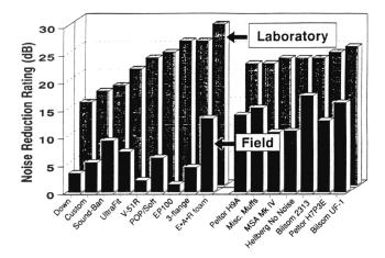
FIGURE G-1 Comparison of hearing protection device NRRs by device type: manufacturers' laboratory data versus real-world "field" data. Adapted with permission from Berger (2003), Fig. 10.18, p. 421.
