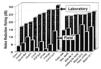
FIGURE 4-3 Comparative noise reduction ratings based on manufacturers' laboratory tests and real-world "field" performance of different types of hearing protection devices. Adapted with permission from Berger, 2003b, Fig. 10.18, p. 421.
