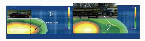
FIGURE 5-18 Acoustic images of typical noise source regions for light vehicles and heavy trucks obtained with acoustic beaming. Source: Adapted from Donavan and Rymer (2009).
