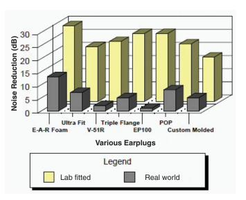
FIGURE 4-2 Comparative noise reduction ratings for various earplugs. Source: NIOSH, 1996.
