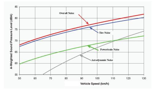
FIGURE 5-17 Typical levels for noise sources in light vehicles. Sources: Adapted from Donavan (1993); Donavan et al. (1998).
