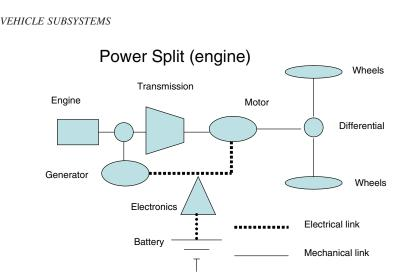
**FIGURE 3-10** Schematic of typical power-split hybrid or plug-in hybrid electric vehicle power-train configuration (such as Prius, Escape, and others).
