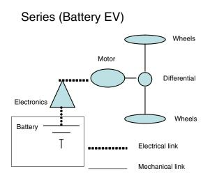
**FIGURE 3-9** Schematic of series drive configuration, battery electric vehicle (EV) (similar to the Nissan Leaf and others).
