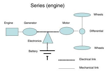
**FIGURE 3-7** Schematic of series drive configuration for a plug-in hybrid electric vehicle (similar to the GM Volt).
