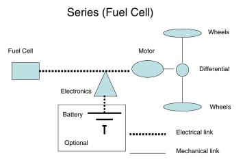
FIGURE 3-8 Schematic of series drive configuration, typical fuel cell vehicle configurations.
