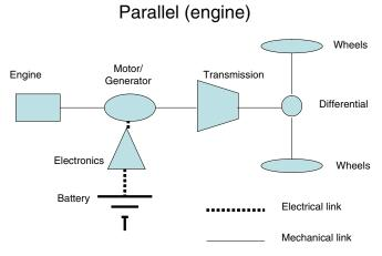
**FIGURE 3-6** Schematic of parallel drive configuration for a hybrid vehicle (similar in concept to the Honda Insight Mercedes S series).
