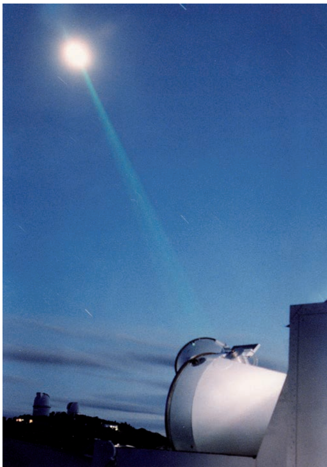
FIGURE 4.4 Lunar laser ranging by the McDonald Laser Ranging System. Lasers are aimed at retroreflectors left on the moon by the Apollo and Lunokhod missions providing range measurements accurate to a few centimeters. SOURCE: Courtesy of R. Ricklefs, McDonald Observatory.
