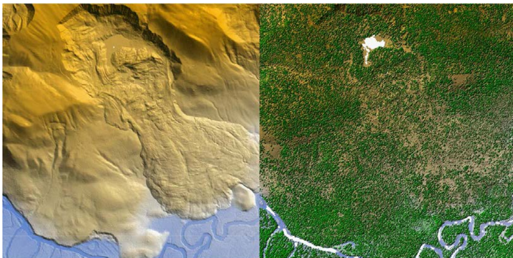
FIGURE 3.7 These false-color geodetic images of a landslide near Flathead Lake, Montana, were made from airborne LiDAR data collected by the NSF National Center for Airborne Laser Mapping (NCALM). Laser shots passed through openings in the forest and reached the ground, allowing a filter to be used to remove the returns from the trees and reveal the landslide, which is not normally visible to the eye or a camera. The white scale bars are 500 meters in length. SOURCE: Ramesh Shrestha, National Center for Airborne Laser Mapping (NCALM), University of Houston; see also Carter et al., 2007.
