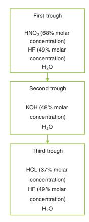
**FIGURE D-3** Flow sheet of chemicals used for the texture preparation (based on discussions with polysilicon production plants in China).
