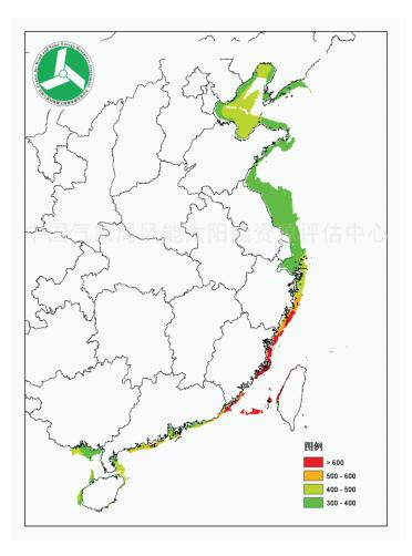
**FIGURE 2-6** Offshore wind power potential by numerical methods at 50 m hub height excluding areas subjected to strong and super typhoons in the past 45 years. Correspondence of wind power density (wind class) is > 600 W/m<sup>2</sup> (> Class 6); 500–600 W/m<sup>2</sup> (Class 5); 400–500 W/m<sup>2</sup> (Class 4); 300–400 W/m<sup>2</sup> (Class 3); 200–300 W/m<sup>2</sup> (Class 2); < 200 W/m<sup>2</sup> (Classes 1 and 0). Source: China Meteorological Administration
