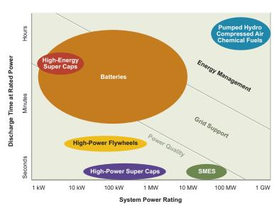
**FIGURE 3-5** Capabilities of a variety of storage technologies. SMES = superconducting magnetic energy storage. Source: NAS/NAE/NRC, 2010a.
