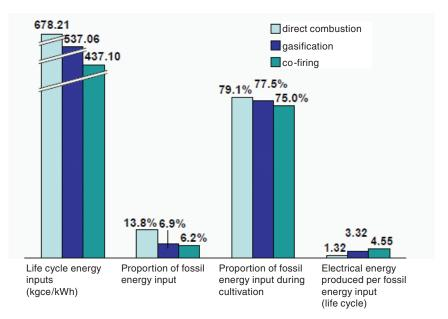
**FIGURE C-4** Relative efficiencies for direct-combustion, gasification, and biomass cofiring power plants.
