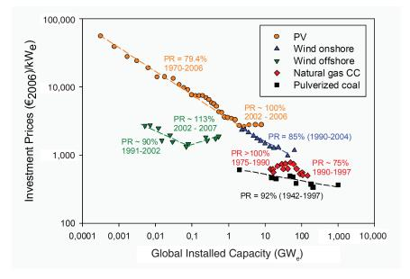
**FIGURE 5-5** Comparison of experience curves for various energy supply technologies. Source: Junginger et al., 2008. Reprinted with permission.
