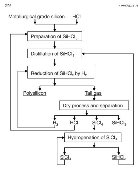
FIGURE D-1 Flow sheet of the modified Siemens process.
