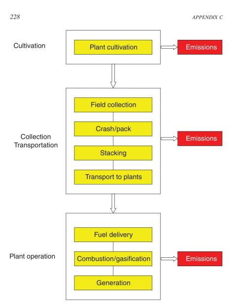
FIGURE C-1 Process flow-diagram of biomass combustion for electricity.
