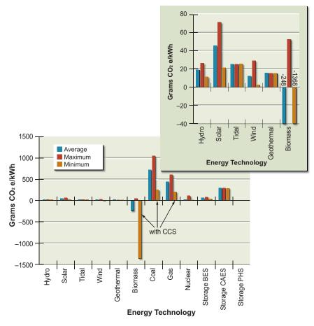
**FIGURE 4-2** Life cycle emissions of greenhouse gases (in CO<sub>2</sub> equivalents) for various sources of electricity. Source: NAS/NAE/NRC, 2010a.
