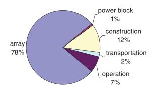
**FIGURE B-3** The percentage breakdown of  $CO_2$  emissions in the life cycle of solar thermal power plants.
