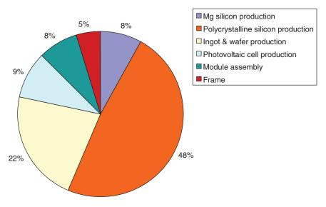
**FIGURE 4-6** Breakdown of energy use in multicrystalline silicon PV module manufacturing. Adapted from estimates provided by Alsema (2000) and Alsema and de Wild-Scholten (2006).
