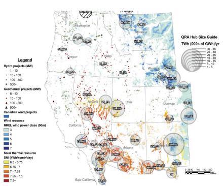
**FIGURE 2-16** QRAs showing potential for electricity generation from a variety of renewable sources (biomass is not shown; only some part of the Canadian QRAs shown). Maps like this one were the first step in planning for renewable electricity and new transmission and distribution on a regional basis with input from the public. Source: WGA, 2009.
