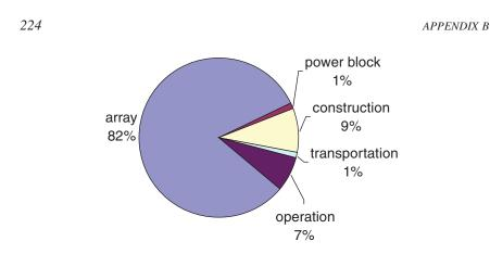
**FIGURE B-2** The percentage breakdown of energy demand in the life cycle of solar thermal power plants.
