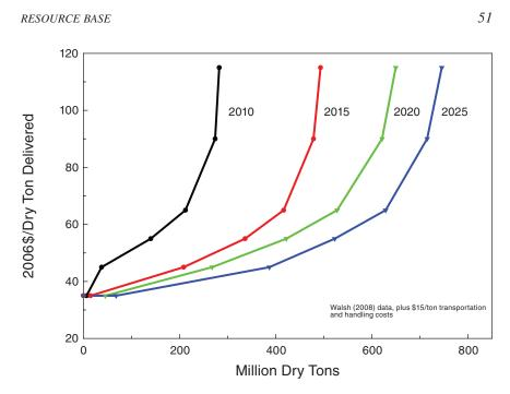
**FIGURE 2-12** Biomass supply curves indicating how much feedstock can be delivered to a conversion facility at a certain price for various scenarios from today to 2025. Source: Walsh, 2008 (plus \$15/ton transportation and handling costs).
