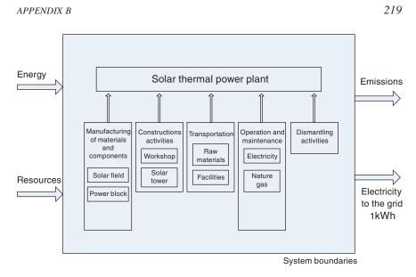
FIGURE B-1 Life cycle of a solar thermal power plant.
