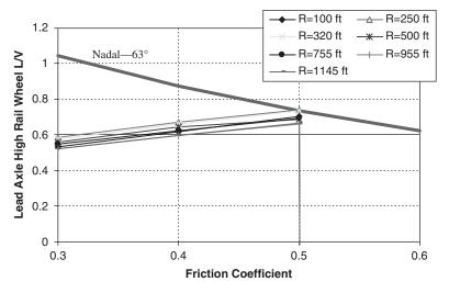
*Figure 29.* Wheel L/V ratio, Type 1 transit rail car, perturbation Level 3, 15 mph, worn rail.
