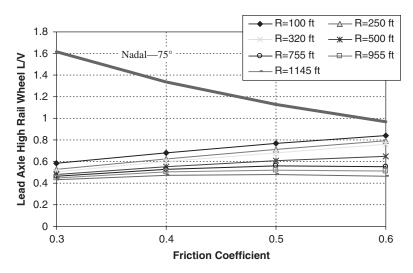
*Figure 34. Wheel L/V ratio, Type 1 light rail vehicle, steady-state curving, 15 mph.*
