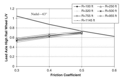
Figure 24. Wheel L/V ratio, Type 1 transit rail car, Level 3 perturbations 15 mph, no guard rail.
