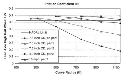
*Figure 25. The wheel L/V ratio of a Type 1 transit rail car with a 0.6 friction coefficient and a 63° flange angle.\**
