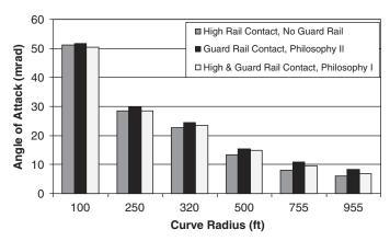
Figure 9. The axle AOA of a Type 1 transit rail car with a guard rail.
