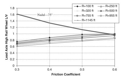
*Figure 35.* Wheel L/V ratio, Type 1 light rail vehicle, Level 3 perturbations, 15 mph.
