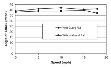
Figure 10. Measured transit rail car leading axle AOA on TTL track.
