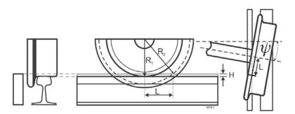
Figure 6. Wheel back/restraining rail contact.
