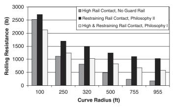
Figure 12. The vehicle rolling resistance of a Type 1 transit rail car with a restraining rail.
