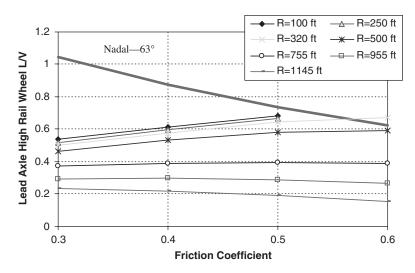
*Figure 27.* Wheel L/V ratio, Type 1 transit rail car, steady-state curving, 15 mph, worn rail.
