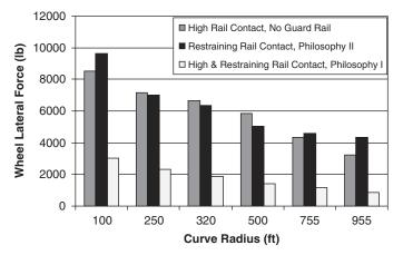
*Figure 11. The wheel lateral force of a Type 1 transit rail car with a restraining rail.*
