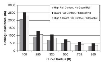
Figure 16. The vehicle rolling resistance of a Type 1 light rail vehicle with a guard rail.
