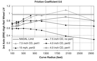
*Figure 39.* Wheel L/V ratio, Type 2 light rail vehicle, friction coefficient 0.6.
