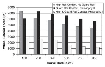
*Figure 15. The wheel lateral force of a Type 1 light rail vehicle with a guard rail.*
