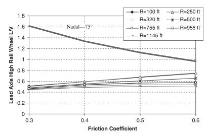
*Figure 37. Wheel L/V ratio, Type 2 light rail vehicle, steady-state curving, 15 mph.*
