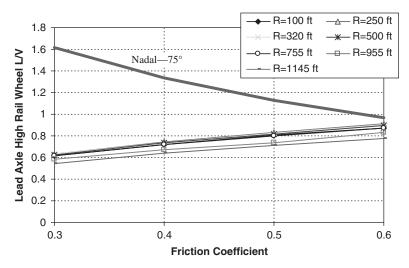
*Figure 38.* Wheel L/V ratio, Type 2 light rail vehicle, Level 3 perturbations, 15 mph.
