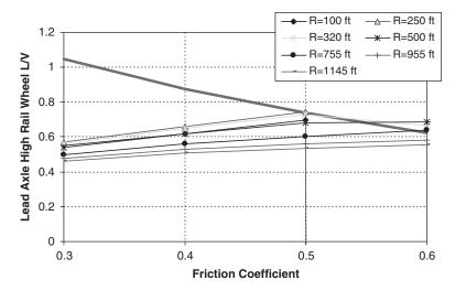
*Figure 28. The wheel L/V ratio, Type 1 transit rail car, perturbation Level 1, 15 mph, worn rail.*
