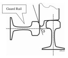
Figure 7. Wheel and horizontal guard/restraining rail installed at a low position.
