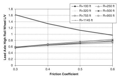
*Figure 31.* Wheel L/V ratio, Type 1 transit rail car, 15 mph, 75° flange angle, perturbation Level 2.
