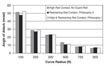
Figure 14. The axle AOA of a Type 1 transit rail car with a restraining rail.
