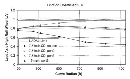
Figure 33. Wheel L/V ratio, Type 1 transit rail car, 75° flange angle, friction coefficient 0.6.\*
