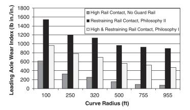
Figure 13. The wear index of a Type 1 transit rail car with a restraining rail.
