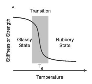
Figure C2.1 Effect of temperature on the properties of polymer composite materials (Zureick and Kahn, 2001)
