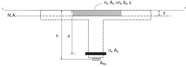
Figure B11-Equivalent FRP transformed section
