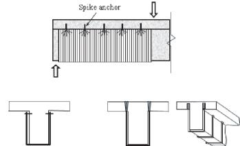
Figure 3.8. Jacketing with anchorages.
