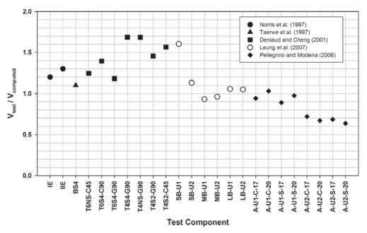
*Figure 3.10.* Scatter of computed strength of reinforced concrete beams with *U*-jacket FRP reinforcement.
