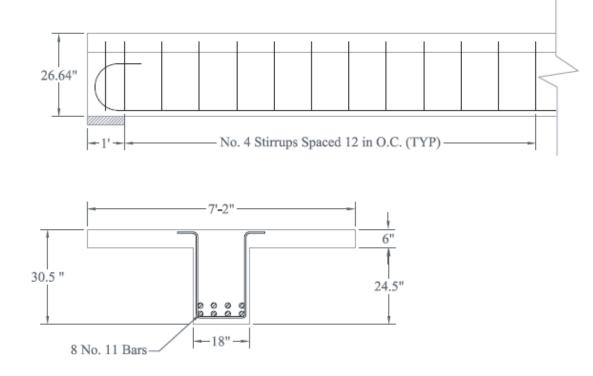
Figure B-12 Beam geometry and reinforcement
