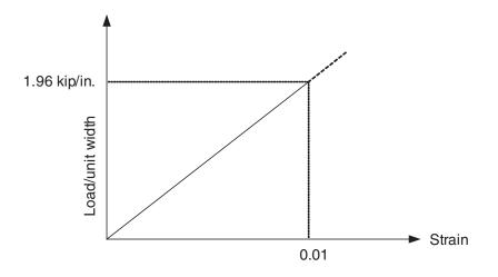
Figure B-1 Load-strain relationship of the FRP reinforcement
