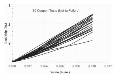
Figure 2.2. Load-strain relation for a field-manufactured composite system (not to failure).
