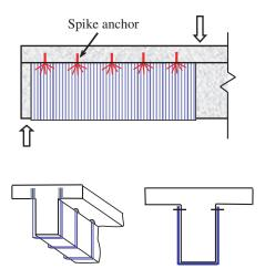
Figure C 4.2-3 Jacketing with anchorages
