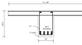
Figure B-4 Reinforced Concrete T-Beam
