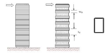
Figure 3.9. Complete wrapping reinforcement.
