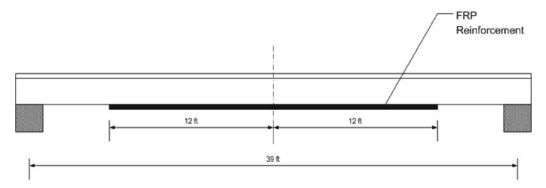
**B-10 FRP reinforcement Detail**
