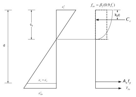
Figure B-8 Strain and stress distribution in the T-beam when tension steel reinforcement yield
