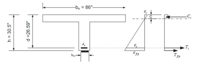
Figure B-6 Reinforced concrete T-beam externally strengthened with FRP reinforcement
