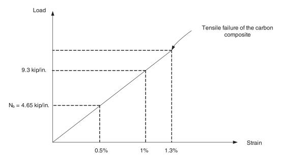
Figure B-3 FRP reinforcement stress-strain diagram for design purposes
