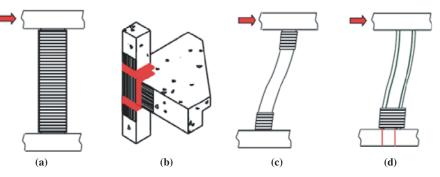
Figure 3.11. Seismic strengthening examples: (a) shear strengthening of RC column, (b) strengthening of beam-column joint, (c) local confinement in flexural plastic hinge regions, and (d) local confinement at lap splices.
