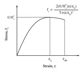
*Figure 3.3. Stress-strain relationship for concrete.*
