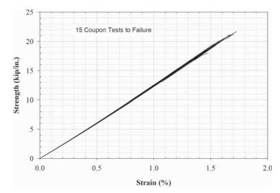
*Figure 2.1. Load-strain relation for shop-manufactured composite system.*
