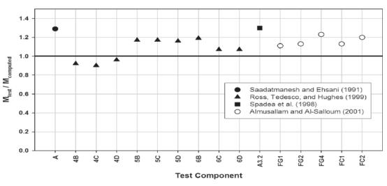
*Figure 3.1. Ratios of test to computed flexural strength for crushing of concrete in compression.*
