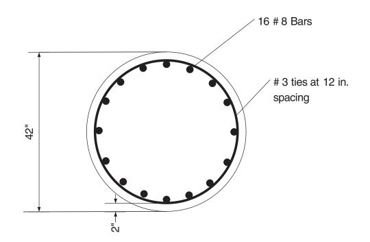
Figure B-14 Reinforcement details of a circular column
