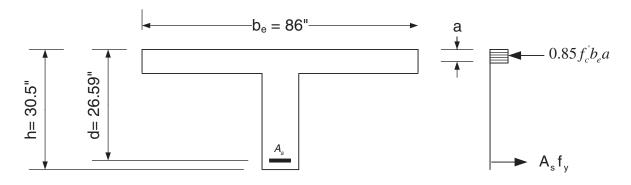
Figure B-5 Force equilibrium on a reinforced concrete T-beam
