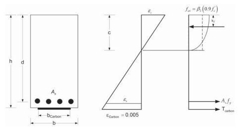
*Figure 3.4. Strain and force diagrams for a reinforced concrete rectangular section.*
