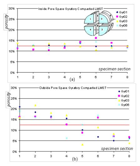
Figure 4-3- Pore space distribution in gyratory compacted limestone (LMST) specimens (a) inside porosity (b) outside porosity
