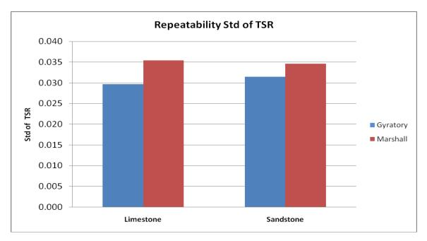
Figure 3-10- Comparison of the within-laboratory standard deviation of TSR values of gyratory and Marshall compacted limestone and sandstone specimens
