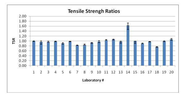
Figure 3-2- Average TSR values of gyratory compacted limestone mixtures
