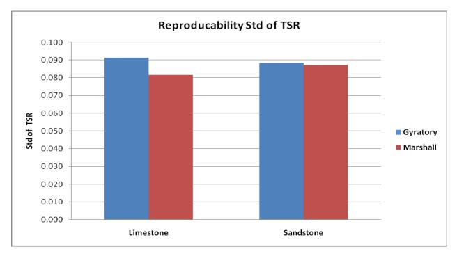
Figure 3-11- Comparison of the between-laboratory standard deviations of TSR values of gyratory and Marshall compacted limestone and sandstone specimens
