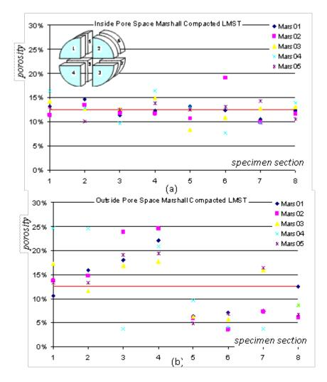
Figure 4-4- Pore space distribution in Marshall compacted limestone (LMST) specimens (a) inside porosity (b) outside porosity
