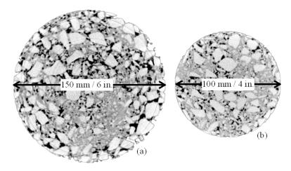
Figure 4-1- Typical X-ray tomography images of 6" gyratory and 4" Marshall compacted specimens
