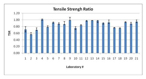
Figure 3-6- Average TSR values of gyratory compacted sandstone specimens
