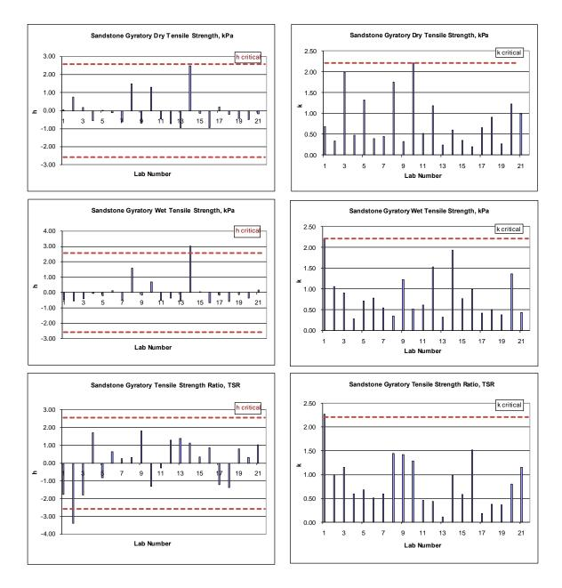
Figure D-1- h and k statistics of indirect tensile strength properties of sandstone gyratory specimens
