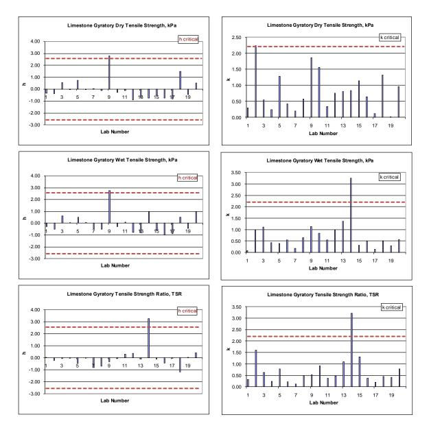
Figure B-1- h and k statistics of indirect tensile strength properties of limestone gyratory specimens
