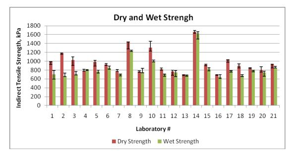
Figure 3-5- Average dry and wet indirect tensile strength values of gyratory compacted sandstone specimens
