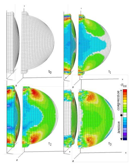
Figure 4-7- Finite element continuum analysis of dry indirect tension test
