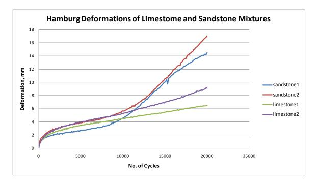
Figure 2-1- Deformation of limestone and sandstone mixture in Hamburg wheel tracking test
