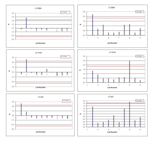
Figure B-2: h and k consistency statistics of length measurements of 4"cores
