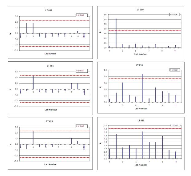
Figure B-1: h and k consistency statistics of length measurements of 6"cores
