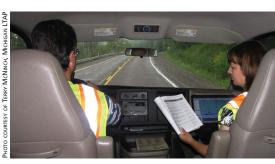
A driver and passenger log data in a Pavement Surface Evaluation and Rating (PASER) survey. Road surveying is one of TAMC's four strategic initiatives.
