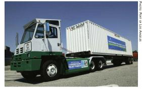
As part of its green terminal program, in 2009 the Port of Los Angeles purchased 20 electric, heavy-duty trucks capable of hauling 30-ton shipping containers in and around the San Pedro Bay port complex.
