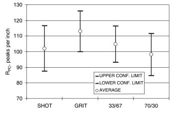
**Figure 7** Average values and 95 percent confidence ranges for  $R_{PC}$  profilometer data on A36 panels prepared with different abrasive mixes.
