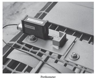
Figure 3 Surface profile gauges.
