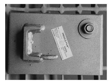
Figure 2 Testex<sup>TM</sup> tape to evaluate surface profile.
