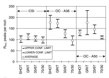
**Figure 8**  $R_{PC}$  versus abrasive mix and applicator.
