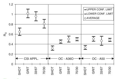
Figure 9 Values of R<sub>o</sub> versus abrasive mix and applicator.
