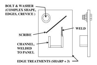
Figure 1 Test panel used for corrosion testing.
