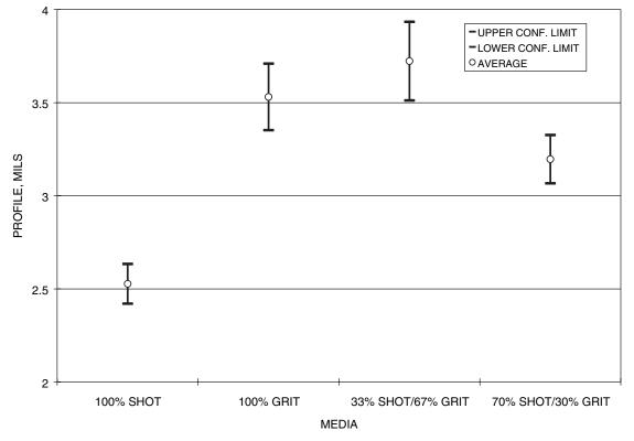
Figure 5 Testex<sup>™</sup> replica tape profile ranges (CSI-prepared test panels).
