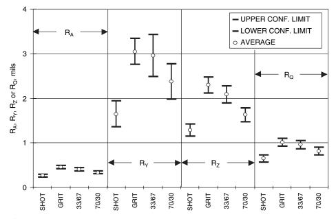
**Figure 6** Average values and 95 percent confidence ranges for  $R_A$ ,  $R_Y$ ,  $R_Z$ , and  $R_Q$  profilometer data on A36 panels prepared with different abrasive mixes.
