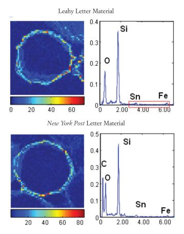
**FIGURE 4-1** SEM of Leahy and *New York Post* powders. SOURCE: SNL. This figure is the work of Sandia National Laboratories, taken or made during the course of an employee's official duties. As a work of the U.S. federal government, the image is in the public domain.
