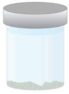
**FIGURE 5.C.1** Example of static container for PCT. SOURCE: Eric Pierce, Oak Ridge National Laboratory.
