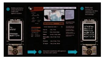
FIGURE 9 Example of requesting and receiving real-time transit information by means of SMS.
