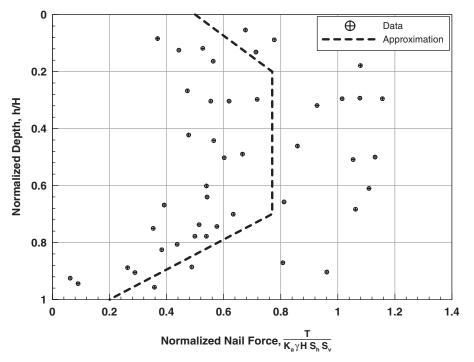
Figure 3-30. Summary of tensile forces measured in instrumented SNWs.
