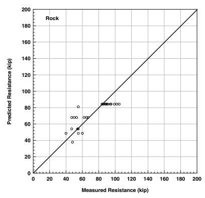
Figure 3-25. Measured and predicted pullout resistance—rock.
