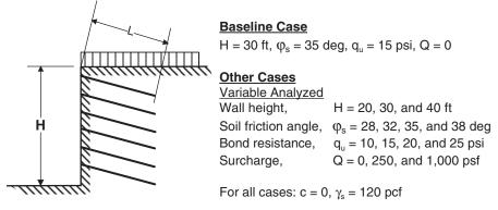
Figure D-2. Geometry of SNW in comparative analyses.
