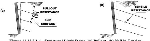
Figure 11.12.5.1-1 Structural Limit States: (a) Pullout; (b) Nail in Tension
