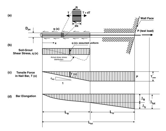
Figure 3-21. Loads and elongation in a soil nail load test.
