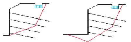
Figure D-1. Slip surfaces used in SNAIL: (a) two wedges through toe and (b) two wedges under toe.
