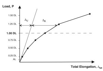
Figure 3-22. Reduction of soil nail load-test data.
