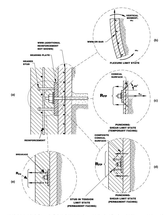
Figure 11.12.6.1-1 Limit States in Soil Nail Wall Facings: (a) Typical Section; (b) Flexure; (c) Punching-Shear in Temporary Facing; (d) Punching-Shear in Permanent Facing; and (e) Headed-Stud in Tension
