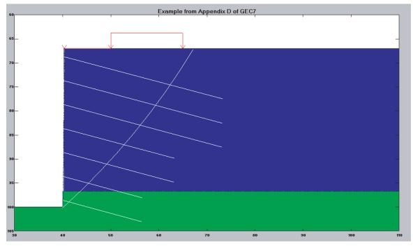
Figure D-5. Critical failure surface calculated using GOLDNAIL.
