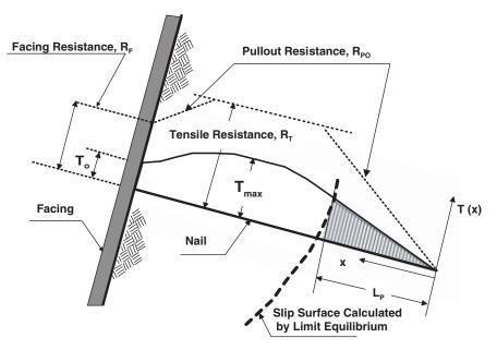
Figure 3-9. Schematic representation of structural resistances.
