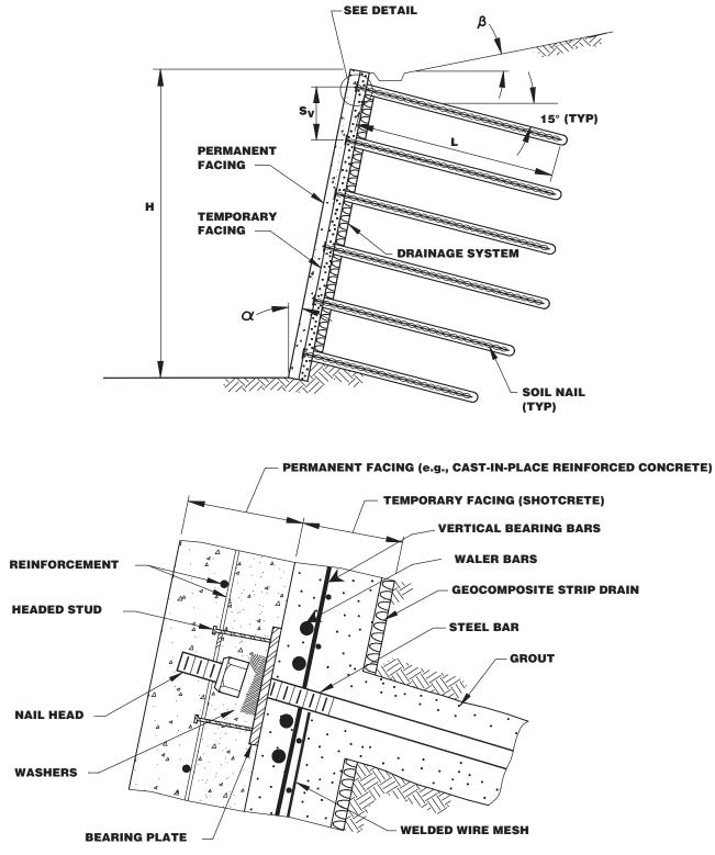
Figure 3-4. Typical cross section of a soil nail wall in common U.S. practice.
