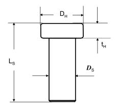
Figure 11.12.6.4-1 Geometry of a Headed-Stud
