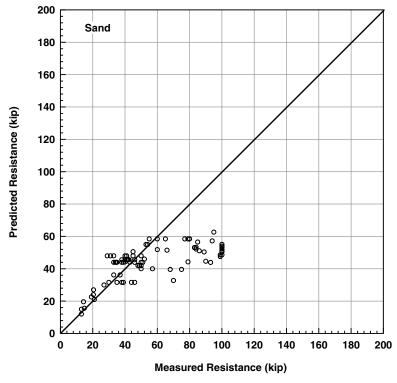
Figure 3-23. Measured and predicted pullout resistance—sand.
