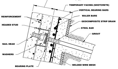
Figure 11.12.1-1 Soil Nail Wall : (a) Typical Section, (b) Nail Head and Facing Details
