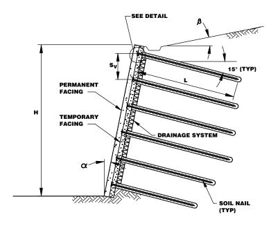
/-- PERMANENT FACING (e.g., CAST-IN-PLACE REINFORCED CONCRETE)
