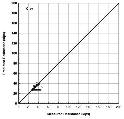
Figure 3-24. Measured and predicted pullout resistance—clay.
