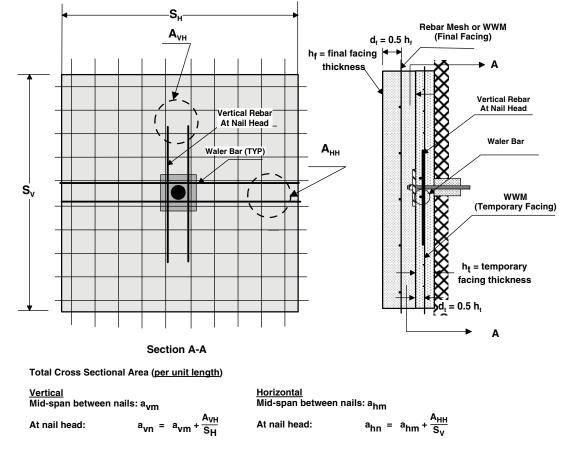
Figure 3-12. Resistance and reinforcement nomenclature for flexure limit state.
