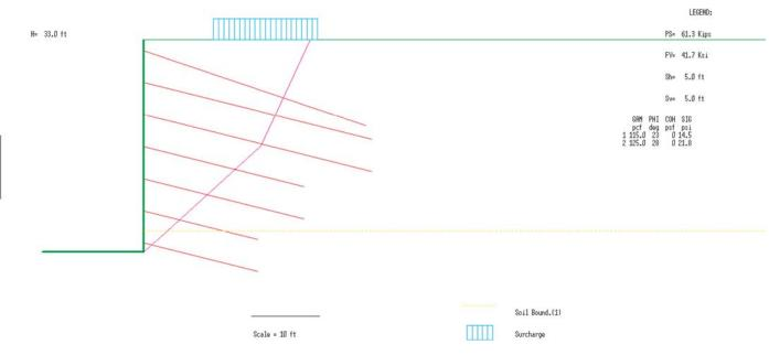
Figure D-6. Critical failure surface calculated using SNAILZ.
