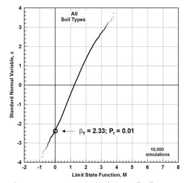
Figure 3-40. Monte Carlo simulation—all soil types.
