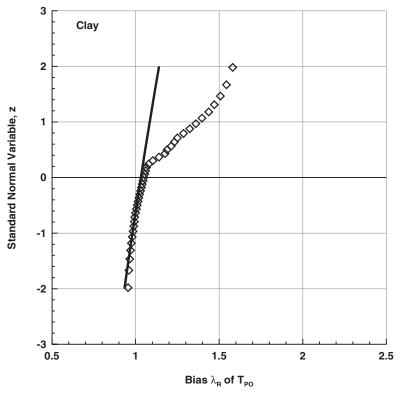
Figure 3-27. Bias  $\lambda_R$  of pullout resistance—clay.
