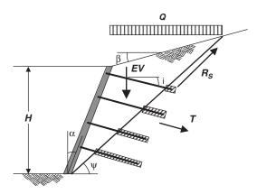
Figure 3-6. Main forces in overall stability.
