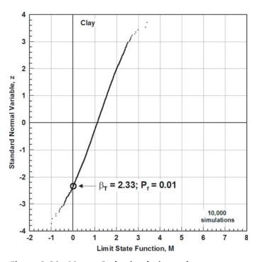
Figure 3-38. Monte Carlo simulation—clay.
