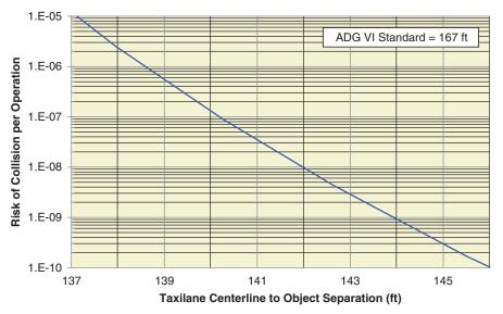
Figure AA-27. Collision risk associated with taxilane to object separation for ADG VI.
