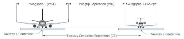
Figure A-2. Example of taxiway/taxiway separation analysis for specific aircraft.
