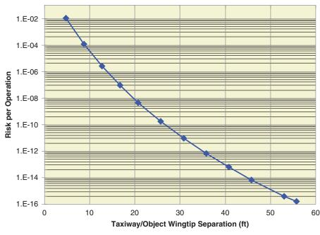
Figure 13. Taxiway/object collision probability based on wingtip separation.
