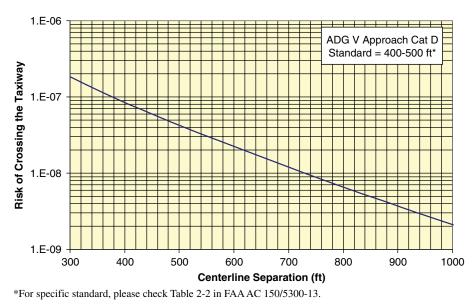
Figure AA-45. Landing veer-off collision risk for ADG V.
