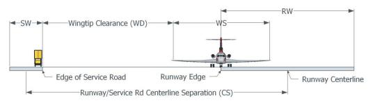
Figure A-12. Typical runway/object scenario for runway veer-off incidents.
