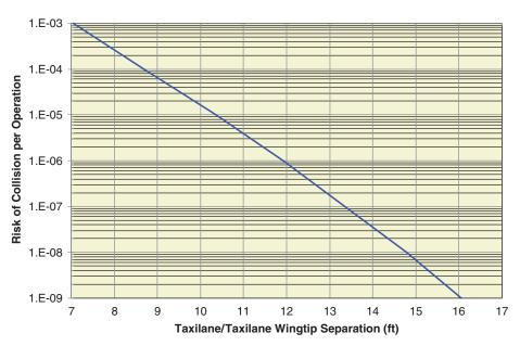
*Figure 14. Taxilane/taxilane collision probability based on wingtip separation.*
