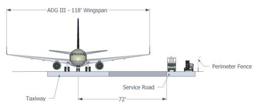
Figure A-6. Example of analysis for taxiway/object separation.
