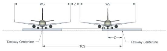
Figure 6. Parallel taxiway separation geometry.
