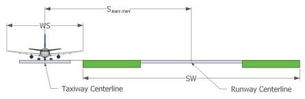
Figure 5. Runway/parallel taxiway separation distance.
