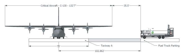
Figure H-18. Cross-section of the existing separation at ILG.
