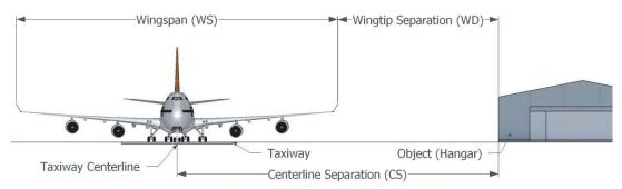
Figure A-5. Example of taxiway/object separation analysis for specific aircraft.
