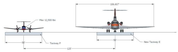
Figure H-17. Cross-section of the existing parallel taxiway separation at ACK.
