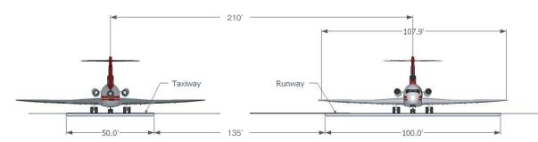
Figure H-13. Cross-section of the existing runway/taxiway separation at LCI.
