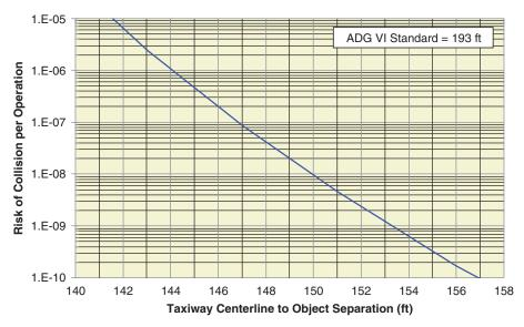
*Figure AA-13.* Collision risk associated with taxiway to object separation for ADG VI.
