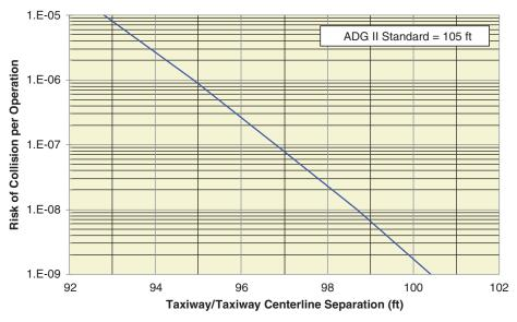
*Figure AA-2.* Collision risk associated with taxiway centerline separation for ADG II.
