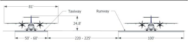
Figure H-12. Cross-section of the runway/taxiway existing separation at HYA.
