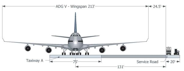
Figure H-10. Cross-section of the existing separation at ORD for Case Study # 10.
