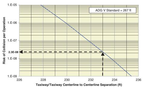
Figure A-4. Example of analysis of taxiway/taxiway separation (ADG V).
