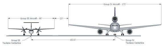
Figure H-1. Cross-section of existing separation at PHL.
