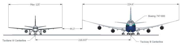
Figure H-15. Cross-section of the existing separation at SEA for Case Study # 15.
