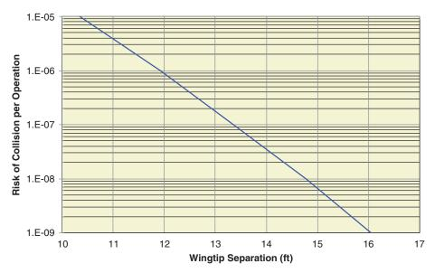
*Figure AA-21.* Collision risk associated with taxilane wingtip separation distance (any ADG).
