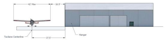
Figure H-6. Cross-section of existing separation at N07.
