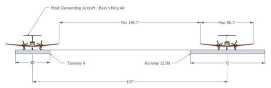
Figure H-20. Cross-section of the existing separation at TAN.
