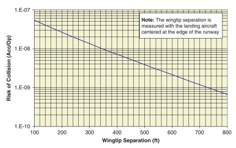
*Figure AA-54. Takeoff veer-off collision risk based on wingtip clearance—any ADG.*
