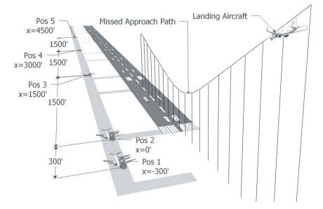
Figure 17. Perspective view of CRM run experiment (not to scale).
