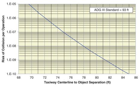
Figure AA-10. Collision risk associated with taxiway to object separation for ADG III.
