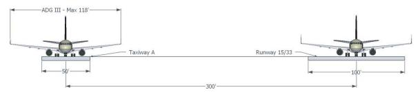
Figure H-3. Cross-section of the existing separation at ADS.
