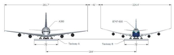
Figure H-7. Cross-section of existing separation at JFK.
