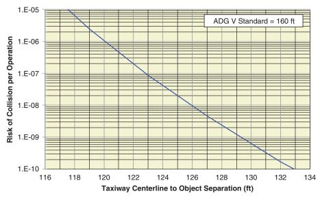
*Figure AA-12.* Collision risk associated with taxiway to object separation for ADG V.
