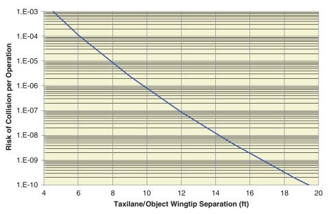
Figure 15. Taxilane/object collision risk based on wingtip separation.
