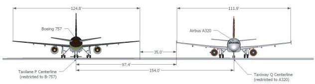
Figure H-9. Cross-section of the existing separation at MSP.
