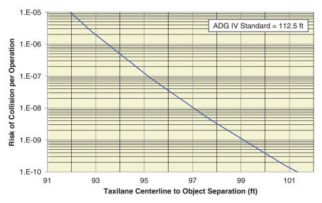
Figure AA-25. Collision risk associated with taxilane to object separation for ADG IV.
