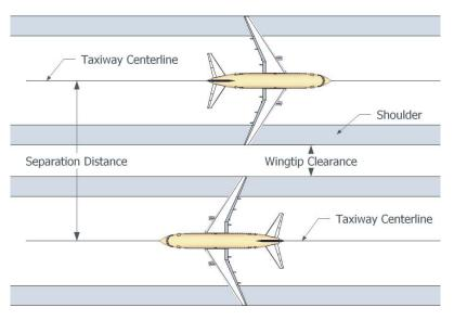
Figure 1. Wingtip clearance, parallel taxiways.
