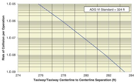
*Figure AA-6.* Collision risk associated with taxiway centerline separation for ADG VI.
