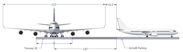
Figure H-8. Cross-section of existing separation at EWR.
