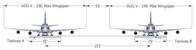
Figure H-11. Cross-section of the existing separation at ORD for Case Study # 11.
