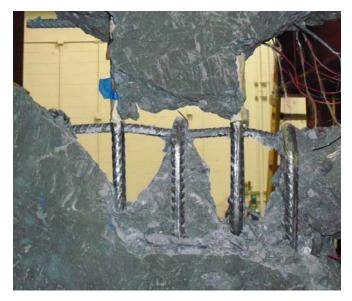
Figure 22 Deformation of lacer bar.
