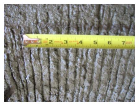
**Figure 13** Intentionally roughened surface, by means of raking, of top web of precast beam used for the construction of Concept 2 laboratory bridge specimen.
