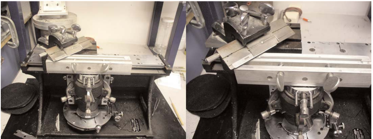
Figure A-5. Edge shaving of BAM test specimens.
