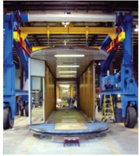
FIGURE 35 Tami-Lift mobile gantry crane.
