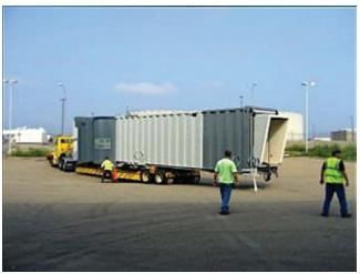
FIGURE 36 Truck delivery of a passenger boarding bridge for overhaul.
