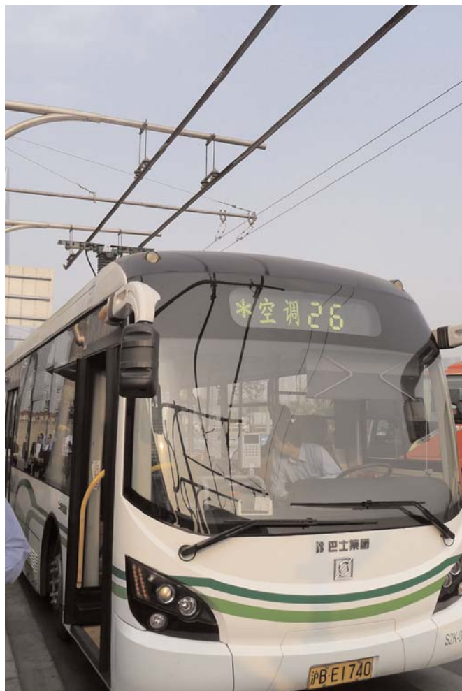
Figure 9 Shanghai's super-capacitor bus combines conventional batteries with super-capacitor technology.
