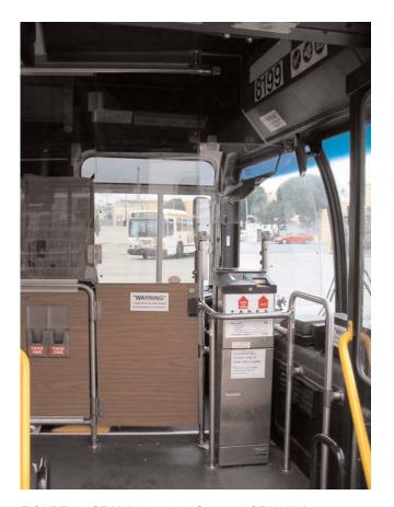
FIGURE 15 SF MUNI barrier. (Courtesy: SF MUNI.)
