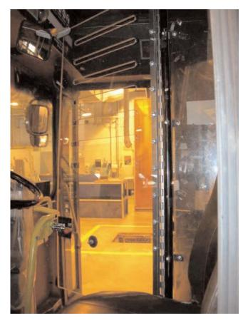
FIGURE 17 Milwaukee County Transit System prototype barrier with slots. (*Courtesy:* Milwaukee County Transit System.)
