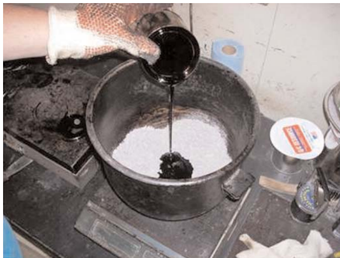
Figure 2. Adding a WMA additive to a mixture in the laboratory.
