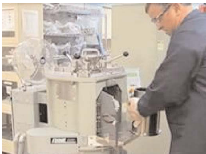
Figure 3. Compacting a WMA specimen in a Superpave gyratory compactor.
