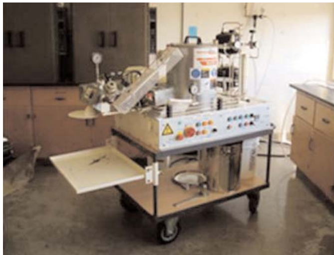
Figure 1. A foaming device for preparing WMA in the laboratory.
