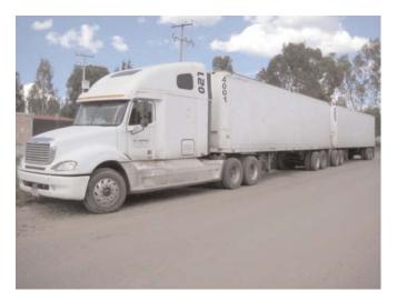
Figure 5 T3-S2-R4 LCV used in Mexico.
