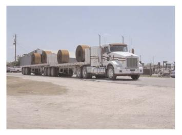
Figure 6 T3-S3-S2 LCV used in Mexico.
