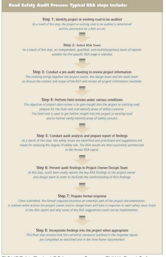
FIGURE 31 Typical RSA steps. *Source: FHWA Road Safety Audit Guidelines (75).*
