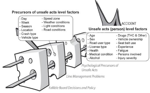
FIGURE 30 Fatal road traffic accident data mapped onto Reason's Swiss Cheese Accident Causation Model. *Source*: Salmon and Lenne (*68*).
