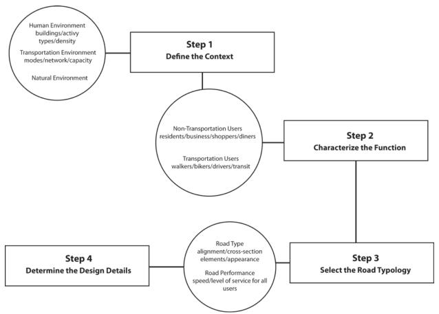
FIGURE 5 Four-step model of highway design process. Source: Garrick and Wang (35).
