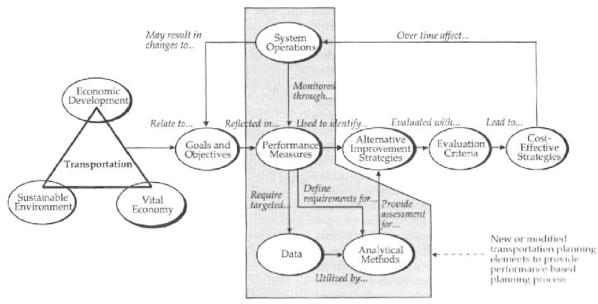
FIGURE 11 Elements of a performance-based planning process. Source: NCHRP Report 446: A Guidebook for Performance-Based Planning (53).
