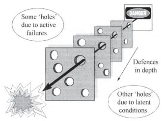
FIGURE 28 Accident trajectory passing through corresponding holes in layers of defenses, barriers, and safeguards. *Source:* Reason (*67*).
