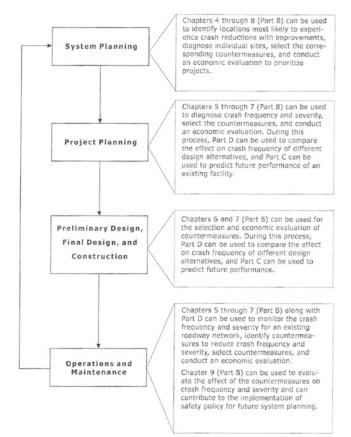
FIGURE 34 Relating the project development process to the *HSM. Source: Highway Safety Manual (71).*
