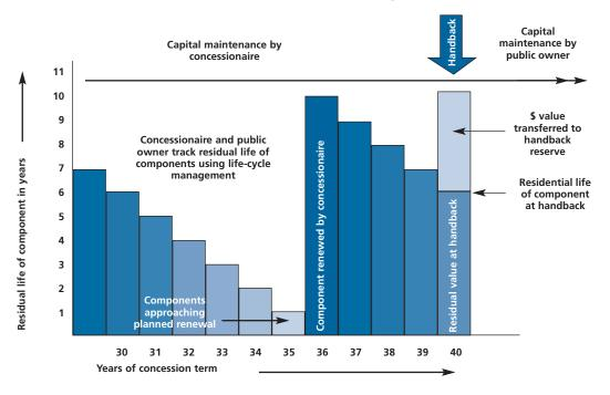
FIGURE 5 Operation of handback reserve for medium service-life elements.
