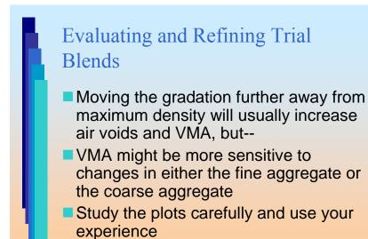
In general, moving the gradation closer to the maximum density gradation will lower VMA, while moving away from the maximum density gradation will increase VMA. Also some specified aggregates will tend to increase VMA, while others will decrease VMA. Experience is the best guide on how specific aggregates will affect VMA.
