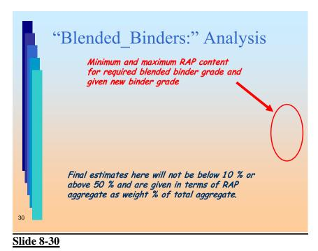
It is assumed that 10 % RAP is the minimum amount that can be accurately added to a mix, so the minimum RAP value given here will not go below 10 %. Similarly, it is assumed that most HMA plants would have trouble adding more than about 50 % RAP to a mix, so the maximum value will not go above 50 %.
