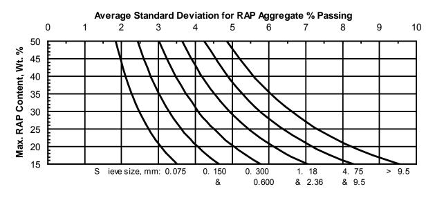
**Figure A3**—Maximum RAP Content as a Function of Average Standard Deviation for Aggregate % Passing, for n = 5 Samples from a Blend of RAP Stockpiles, and No Stockpile Making up More than 70% of the RAP Blend
