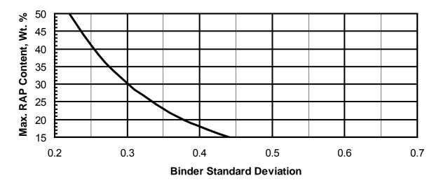
**Figure A2**—Maximum RAP Content as a Function of Standard Deviation for Asphalt Binder Content, for n = 5 Samples from a Single RAP Stockpile
