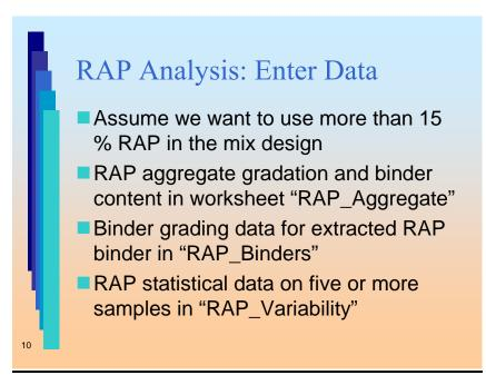
In this part of the example a mix design with RAP is demonstrated. After sampling the RAP, extracting the binder, testing the aggregate and grading the recovered binder, the resulting data is entered in various worksheets in HMA Tools.
