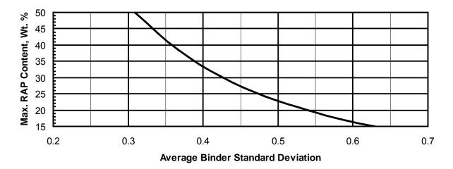
**Figure A4**—Maximum RAP Content as a Function of Average Standard Deviation for Asphalt Binder Content, for n = 5 Samples from a blend of RAP Stockpiles, and No Stockpile Making up More than 70% of the RAP Blend
