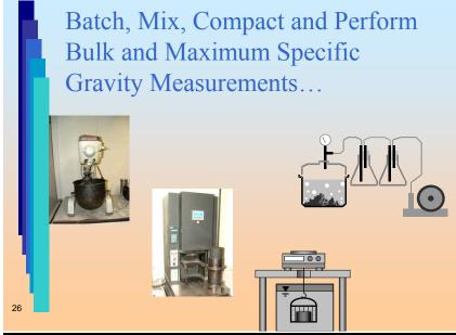
After calculating batch weights, the aggregate and asphalt binder are heated, weighed out, mixed and compacted in a gyratory compactor. Bulk and theoretical maximum specific gravity measurements are then made on the mix.
