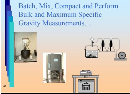
The mix design now proceeds as in the previous example that didn't include RAP. Batches are weighed out, mixed and compacted. Then, bulk and maximum specific gravity values are determined and the volumetric properties compared with the specified requirements.
