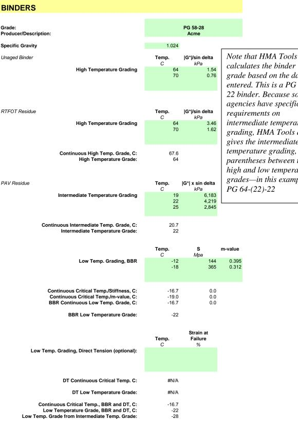
calculates the binder grade based on the data entered. This is a PG 64-22 binder. Because some agencies have specific requirements on intermediate temperature grading, HMA Tools also gives the intermediate temperature grading, in parentheses between the high and low temperature grades—in this example, PG 64-(22)-22
