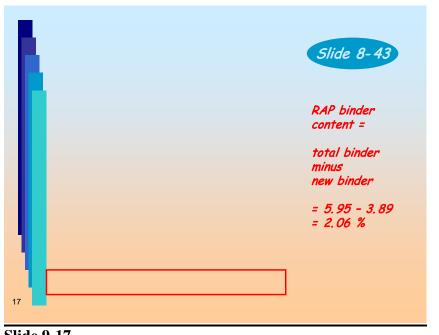
You have to do a little thinking to answer this. This shows slide 8-43, the last slide in Unit 8. The RAP binder content is not shown directly—you have to calculate it by subtracting the new binder content from the total binder content.
