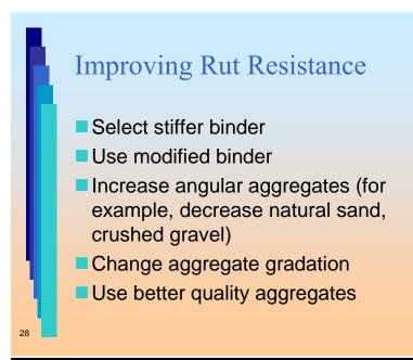
Most mixes designed using this procedure—or the Superpave method should pass the rut resistance test. For those that fail, the first thing to do is to make sure the specimens were prepared properly, that the test was run following the right procedures and that the results were accurately calculated. If the test results seem suspect, repeat the test. If the mix still fails, there are a number of things that can be done to the design to improve rut resistance.
