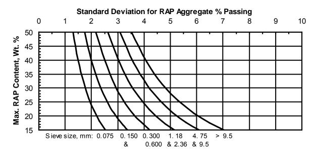
**Figure A1**—Maximum RAP Content as a Function of Standard Deviation for Aggregate % Passing, for n = 5 Samples from a Single RAP Stockpile
