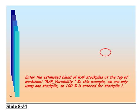
The reliability level should be kept at 80 %. The total of the blends must add up to 100 %. For instance, if you are using two RAP stockpiles, you might enter 50 % for each if you expect to blend them in roughly equal proportions. The estimated maximum RAP content shows zero % because we haven't entered any data on the RAP samples yet.
