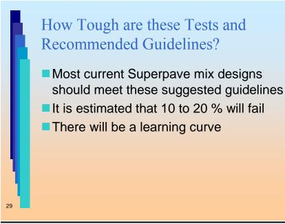
As noted earlier, the test guidelines have been devised so that roughly 80 to 90 % of properly designed mixes will pass.
