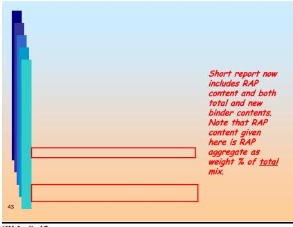
The reports now include RAP content and total and new binder content. The RAP content is slightly different here than when proportioning aggregate blends because the RAP content given here is the RAP aggregate as % by weight of the total mix (not weight % of the aggregate blend).
