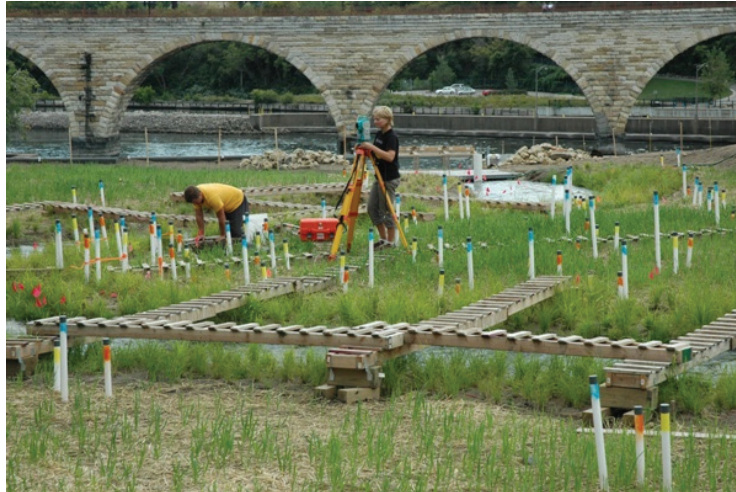
FIGURE 2.21 The Outdoor StreamLab (OSL) facility at the National Center for Earth Surface Dynamics (NCED), located on the banks of the Mississippi River at the University of Minnesota, is dedicated to stream restoration research. OSL uses an abandoned flood bypass channel near St. Anthony Falls to study interactions among river channels, floodplains, and vegetation. Dams and bridge piers can be added to the OSL channel to investigate human-river interactions. SOURCE: Available at http://www.nced.umn.edu/content/outdoor-streamlab-osl . Courtesy of the University of Minnesota.
