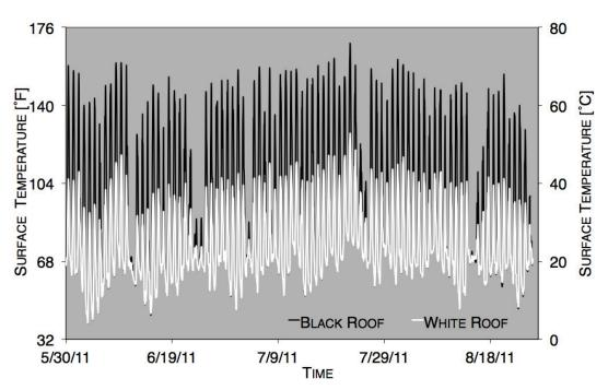
**FIGURE 2.4** The pilot white roof heat island mitigation program in New York City. Results of white vs. black roof surface temperatures. While both colors of roof fluctuate with day and nighttime temperatures, the white roofs stay consistently cooler during the daytime. (*www.nyc.gov/coolroofs*) SOURCE: Gaffin et al., 2012.
