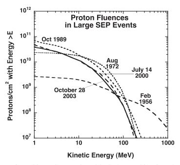
FIGURE 2.6 Energy spectra of several large solar energetic particle (SEP) events. SOURCE: R.A. Mewaldt, C.M.S. Cohen, A.W. Labrador, R.A. Leske, G.M. Mason, M.I. Desai, M.D. Looper, J.E. Mazur, R.S. Selesnick, and D.K. Haggerty, Proton, helium, and electron spectra during the large solar particle events of October-November 2003, *Journal of Geophysical Research* 110:A09S18, 2005. Copyright 2005 American Geophysical Union. Reproduced by permission of American Geophysical Union.
