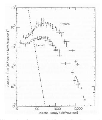
FIGURE 2.1 The observed intensity of cosmic rays at Earth orbit at quiet times. Shown are galactic cosmic-ray protons and helium. The dashed line is a time average of solar energetic particles. SOURCE: J.R. Jokipii, The heliosphere and cosmic rays, Chapter 9 in *Heliophysics—Evolving Solar Activity and the Climates of Space and Earth* (C.J. Schrijver and G.L. Siscoe, eds.), Cambridge University Press, New York, 2010. Copyright © 2010 Cambridge University Press. Reprinted with permission.
