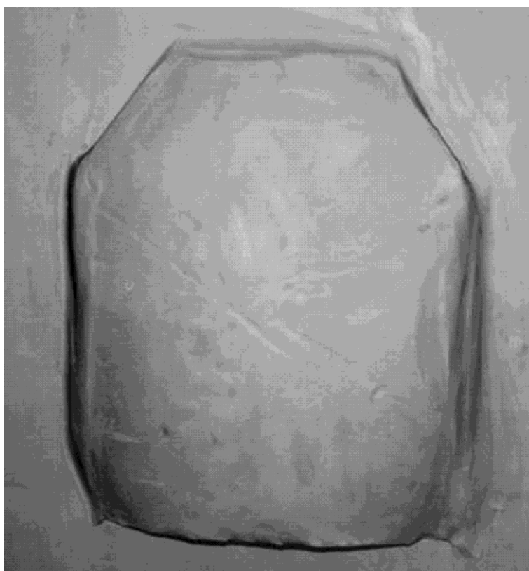
FIGURE 2-1 The clay appliqué applied to the clay box. SOURCE: Richard Sayre, Deputy Director, Office of the Secretary of Defense, Director of Operational Test and Evaluation (OSD DOT&E) Live Fire Test and Evaluation, and Tracy Sheppard, Executive Officer and Staff Specialist, OSD DOT&E Live Fire Test and Evaluation, “DoD In-Brief to the National Research Council Study Team,” presentation to the Body Armor Testing Phase I committee, Aberdeen, Maryland, November 30, 2009.
