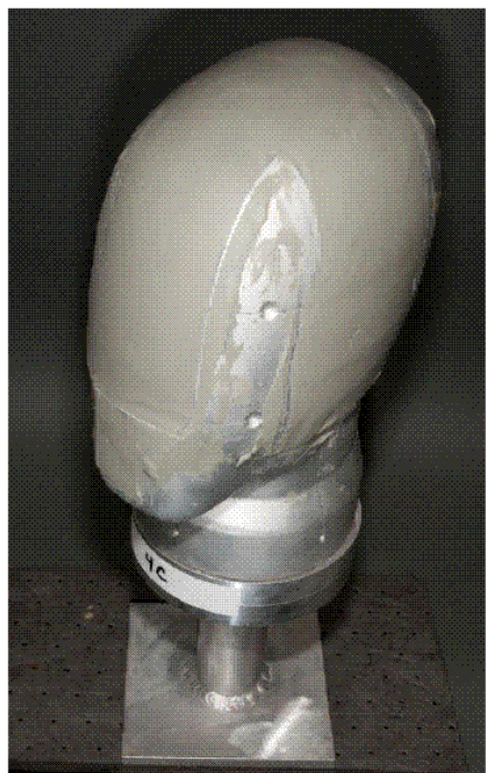
FIGURE 7-11 ATC head form with clay. SOURCE: Rob Kinsler, U.S. Army Research, Development and Engineering Command/ARL.
