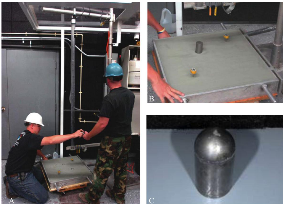
FIGURE 4-3 Column-drop test as performed at ATC. The overall setup is shown in (A). The weight, shown up close in (C), is held in place by an electromagnet at the top of the antiyaw tube. Upon release the weight accelerates under gravity and is implanted into the surface of the modeling clay. The weight is manually removed and the depth of the cavity (two are visible) is measured. Also visible are two thermometer probes used to track the temperature of the modeling clay. The results of a typical drop are shown in (B). Notable is the significant yaw (inclination with respect to the normal of the clay surface). SOURCE: ATC, 2008.
