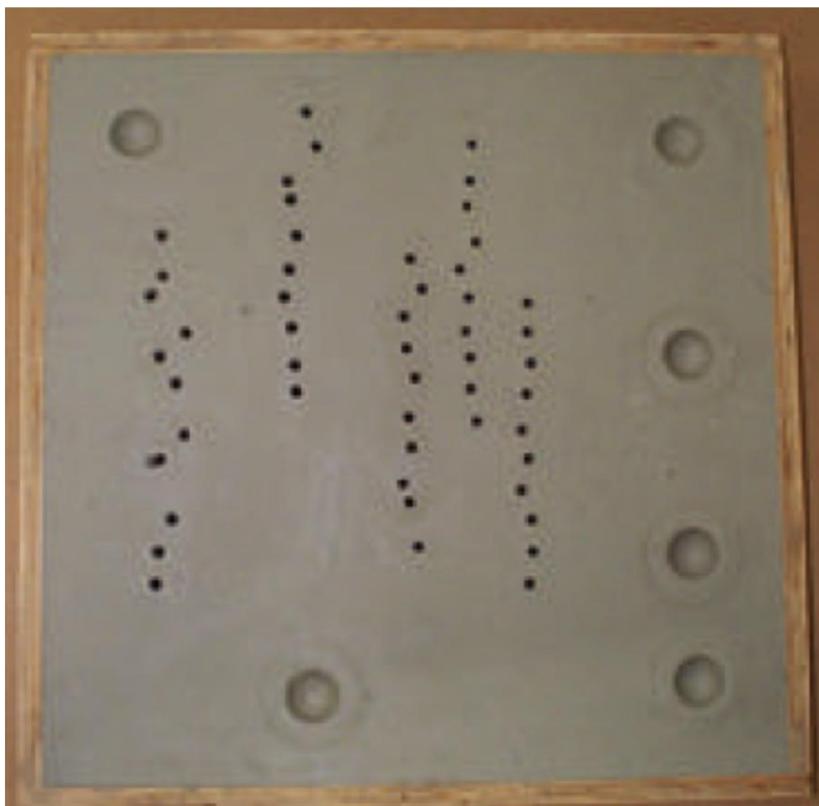
FIGURE 4-8 A clay box used for .32-cal rubber sting ball testing. The large diameter impressions represent NIJ standard calibration drops. SOURCE: Weber, 2000.
