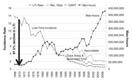
**FIGURE 2-2** Industry safety metrics. For 2007, man-hours are estimated and third-quarter incidence rates are used. (LTI = lost-time incidents; Rec. = recordable; DART = days away and restricted time. SOURCE: IADC 2011.)
