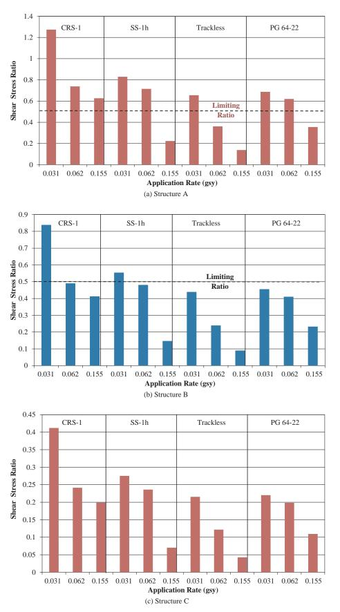
*Figure 79. Calculated shear stress ratios for different tack coat types and residual application rates.*
