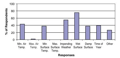
Figure 44. Environmental restrictions on tack application.
