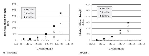
Figure 70. Relationship between ISS and G\*/sin  $\delta$ .
