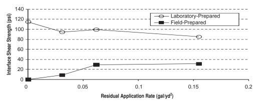
Figure 76. Effects of sample preparation methods on the ISS.
