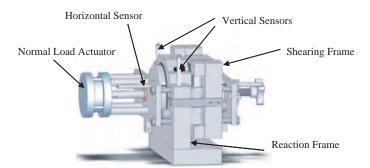
Figure 21. General description of the LISST device.
