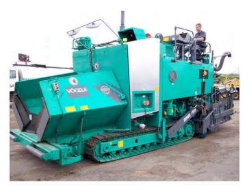
*Figure 23. Asphalt paver with asphalt emulsion tank for tack coat.*
