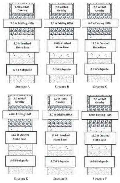
Figure 23. Pavement structures simulated in the FE analysis.
