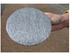
(f) Foam material attachment on loading plate II
