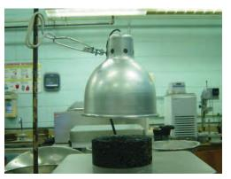
(a) Infrared reflective heating (IRH) lamp.
