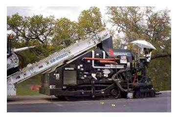
Figure 23a. Roadtec Spray Paver-Spray bar is located at white square between track and screed.
