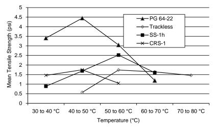
*Figure 54. Variation of the mean tensile strength with temperature.*
