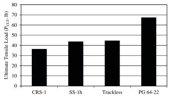
Figure 58. Ultimate tensile load ( $P_{ULT}$ ) for tack coat materials at the softening point.
