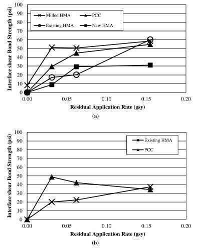
Figure 73. Effects of surface types on ISS for (a) SS-1h tack coat (b) PG 64-22 and (c) trackless tack coat.
