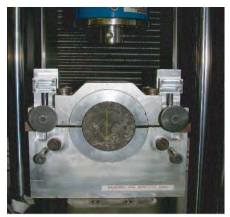
(c) Stabilization of test temperature (30 min.)
