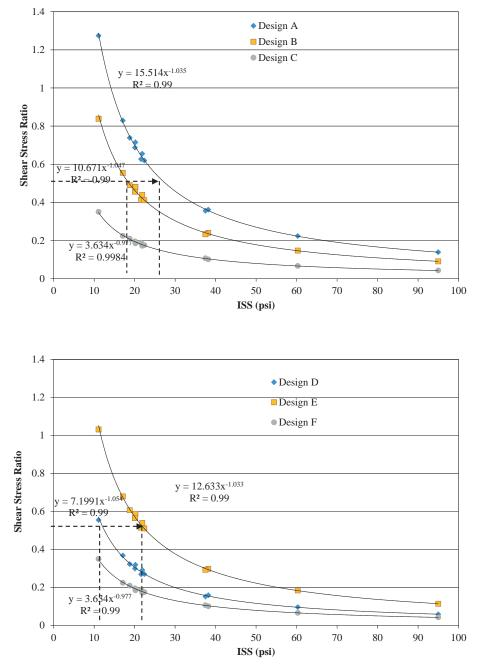
Figure 80. Relationship between shear stress ratio and laboratory-measured ISS.
