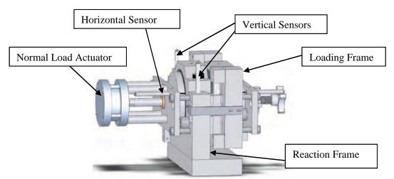
Figure 1. 3-D Illustration Of The Louisiana Interface Shear Strength Tester (LISST) Device.
