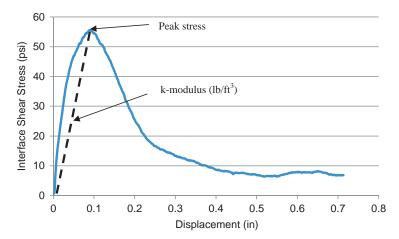
Figure 60. Typical interface shear stress versus displacement for trackless at 0.06 gal/yd<sup>2</sup>.
