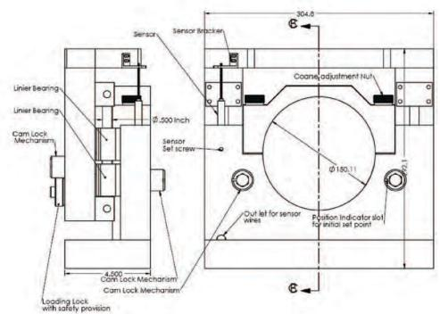
Figure 2. Front and side view of the LISST device.
