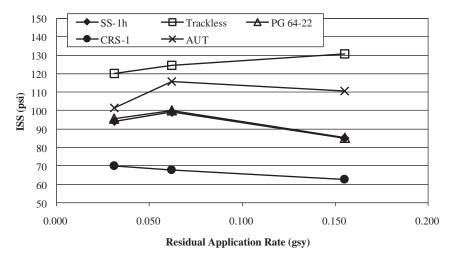
*Figure 75. Effects of residual application rate on ISS for lab-compacted samples.*
