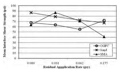
Figure 77. Mean interface shear bond strengths for the OGFC, sand, and SMA mixtures.
