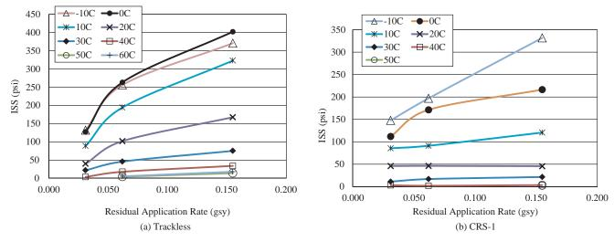
Figure 67. Variation of the ISS with residual application rate and test temperature.
