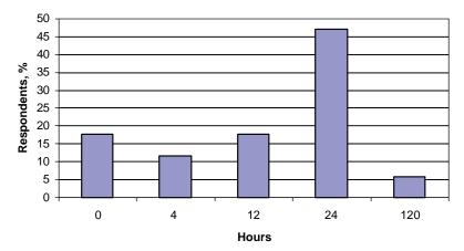
*Figure 40. Time that tack coat can be exposed to traffic before covering with HMA.*
