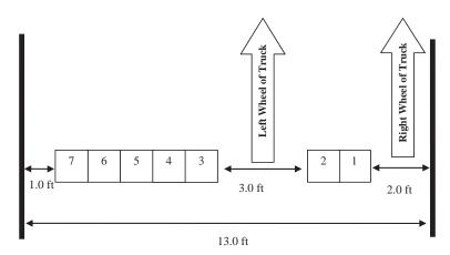
Figure 18. Tack coat rate measurement pad layout for each section.
