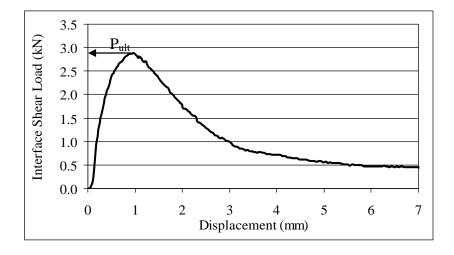
Figure 3. Typical LISST test result.
