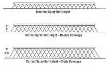
Figure 9. Spray bar height and tack coat coverage.
