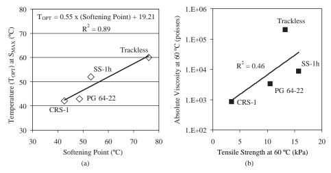
*Figure 57. Relationship between absolute viscosity and softening point and the optimum test temperature.*
