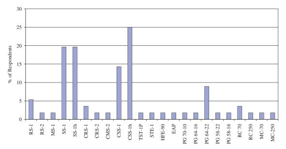
Figure 34. Tack coat materials used on asphalt-treated base.
