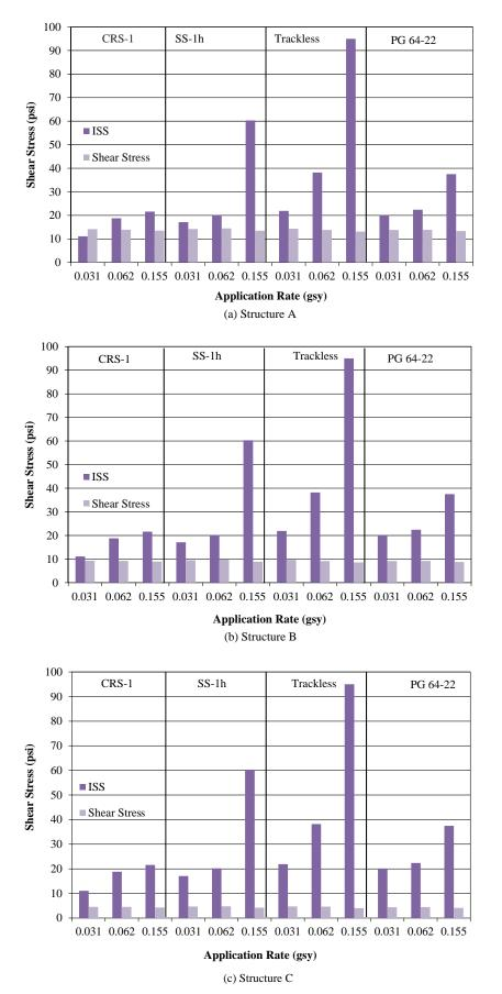
Figure 78. Comparison of the calculated shear stress to the ISS.
