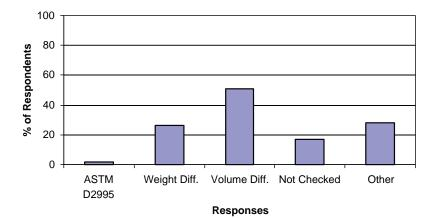
Figure 45. Methods to verify tack application rate.
