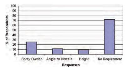
Figure 43. Specified requirements for tack coat application.
