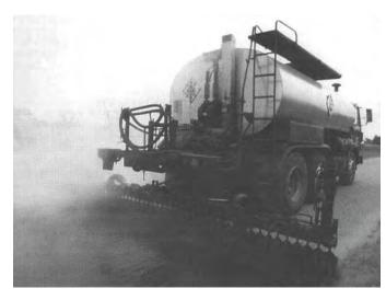
*Figure 4. A typical asphalt distributor (courtesy of Etnyre).*
