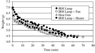
(b) Breaking time of tack coat SS-1h with different heating conditions.
