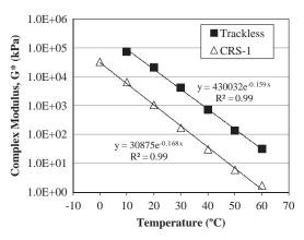
Figure 56. Relationship between complex modulus (G\*) for unaged residues of trackless and CRS-1 and temperature.
