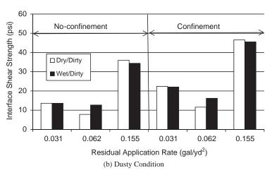
Figure 65. Effect of wetness on ISS for SS-1h tack coat with (a) clean and (b) dusty conditions.
