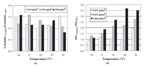
Figure 69. Ratio of trackless to CRS-1 in terms of (a) k-modulus and (b) ISS.
