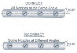
Figure 7. Spray bar nozzle alignment.
