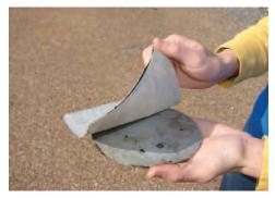
(e) Foam material attachment on loading plate
