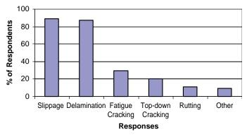
*Figure 49. Failures attributed to improper tack application or type.*
