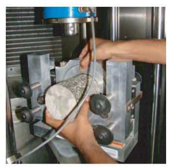
(b) Assemblage of sample and LISST device
