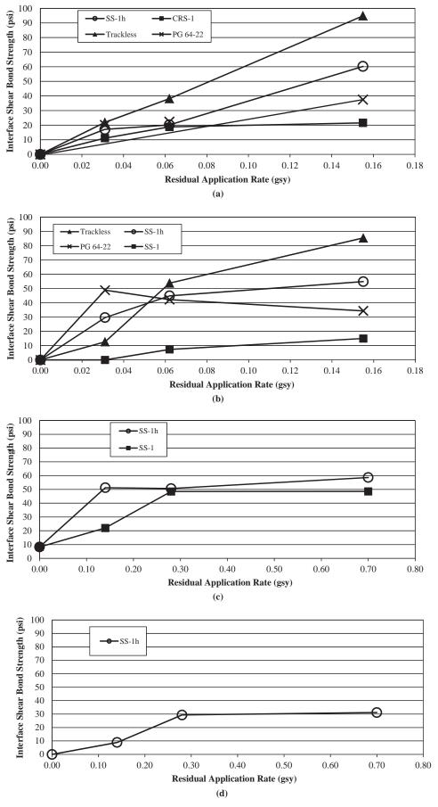
*Figure 72. Effects of residual application rates and tack coat types on ISS for (a) old HMA surface, (b) PCC surface, (c) milled HMA surface, and (d) new HMA surface.*
