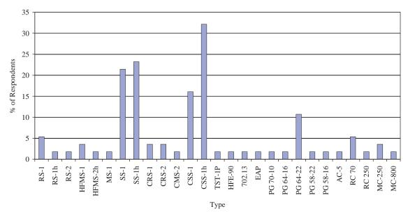
Figure 35. Tack coat materials used on PCC surfaces.
