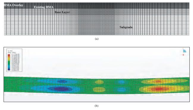
Figure 24. General layout of the FE model (a) and shear stress distribution in the HMA overlay and the old HMA layer (b).
