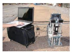
(h) Pull-off testing and data recording
