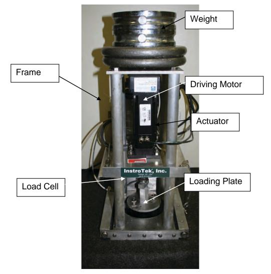
Figure 1. Illustration of the LTCQT device.
