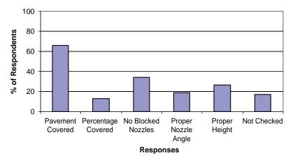
Figure 46. Methods for assurance of tack coverage.
