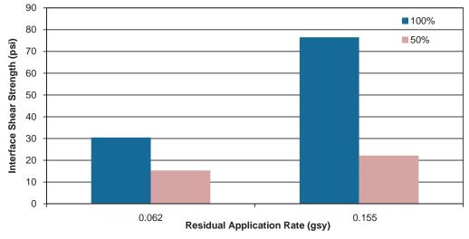
*Figure 66. Effect of tack coat coverage on ISS.*
