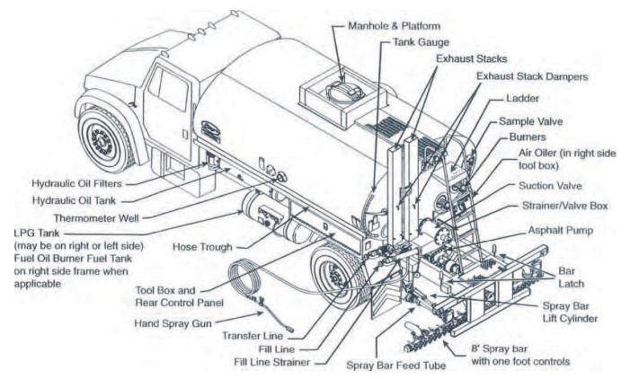
Figure 5. Rear and side component identification for distributor.
