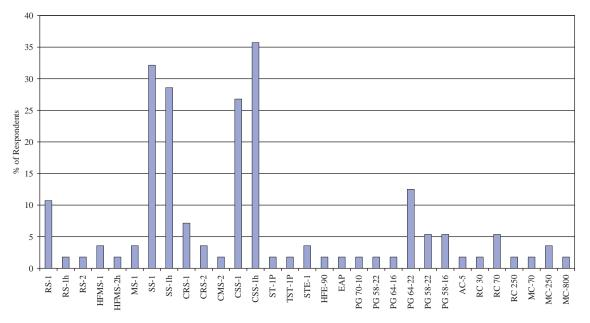
Figure 30. Tack coat materials placed between new HMA layers.
