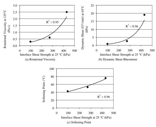
Figure 62. Relationship between ISS with 0.155 gal/yd<sup>2</sup> and rheology test results.
