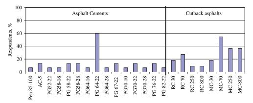
Figure 26. Asphalt cements and cutbacks used as tack coats.
