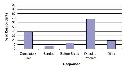
*Figure 42. Methods used to prevent pickup of tack coat by haul trucks.*
