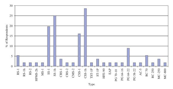
Figure 36. Tack coats used on milled or diamond-ground PCC.
