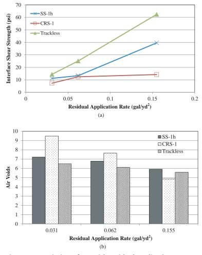
Figure 61. Variation of ISS with residual application rates (a) and variation of air voids with residual application rates: clean and dry condition, no confinement, 25°C (b).
