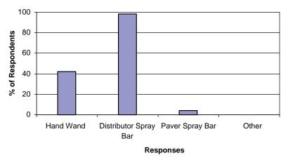
Figure 41. Method for applying tack coat materials.
