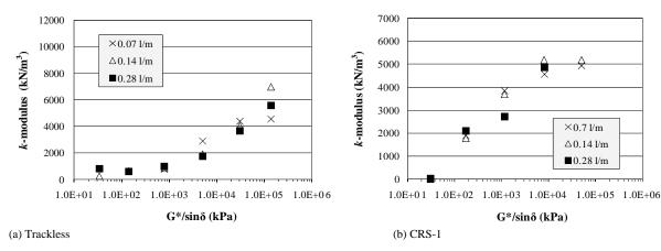
Figure 71. Relationship between k-modulus and G\*/sin  $\delta$ .
