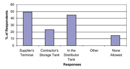
Figure 37. Potential sites for dilution of emulsified asphalt.
