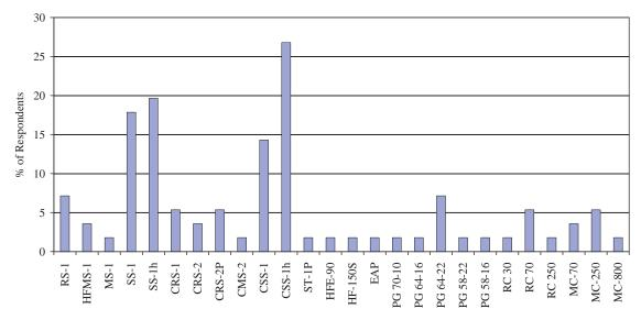
Figure 33. Tack coat materials used on surface treatments, seal coats, or chip seals.
