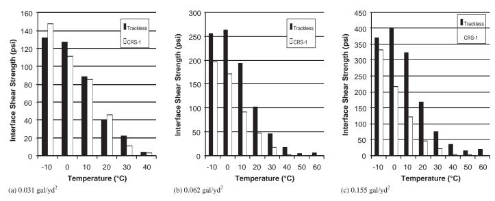
Figure 68. Variation of the ISS with test temperature.
