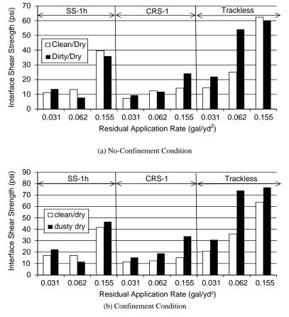
*Figure 64. Dust effect on ISS with (a) no-confinement and (b) confinement.*
