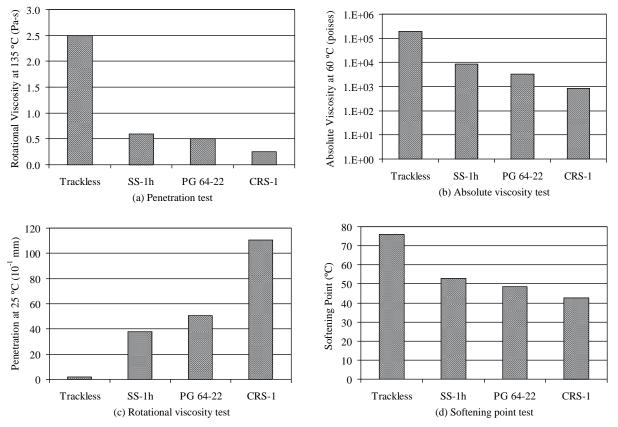
Figure 55. Rheological test results of tack coat materials.
