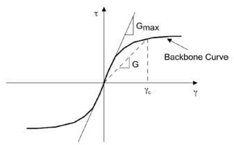
FIGURE 6 Backbone curve as stress-shear strain relationship for monotonic loading.
