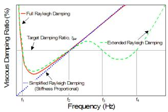
FIGURE 8 Schematic illustration of viscous damping change with frequency (after Park and Hashash 2004).
