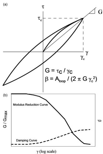
FIGURE 3 Approximation of soil nonlinear behavior (a) Hysteresis loop of soil element loaded by a single cycle of shear strain; (b) Variation of normalized modulus ( $G/G_{max}$ ) and  $\rho$  with shear strain ( $\gamma$ ) (modulus reduction and damping curves).
