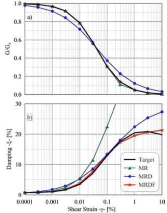
FIGURE 7 Evaluation of proposed damping reduction factor (a) modulus reduction and (b) damping curve using Darendeli's curves for cohesionless soils as target. *Note*:MR = modulus re-matching only with extended Masing rules, MRD = approximate match of both modulus and damping with extended Masing rules, MRDF = modulus reduction and damping matching with non-Masing rules (after Hashash et al. 2010).
