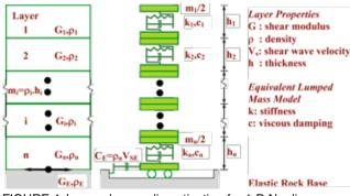
FIGURE 4 Lumped mass discretization for 1-D Nonlinear Hysteretic Site Response Model (Matasovic 1993).
