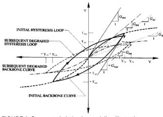
FIGURE 9 Stress-strain behavior modeling illustrating stiffness degradation with the MKZ Constitutive Model (Matasovic 1993; Matasovic and Vucetic 1993).
