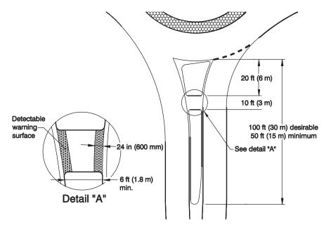
FIGURE 11 Minimum splitter island dimensions (Rodegerdts et al. 2010).
