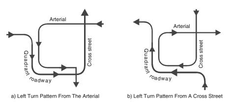
FIGURE 16 Left-turn movements at a QR intersection (based on Hughes et al. 2010).
