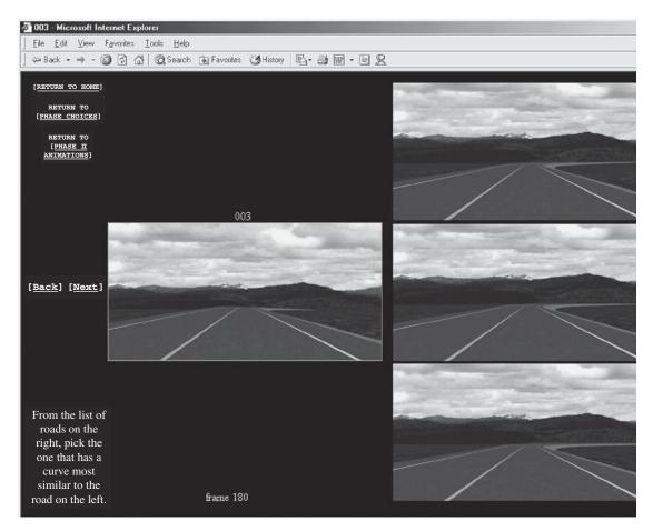
FIGURE 2 Presentation of horizontal curve images for comparison (Hassan et al. 2002).
