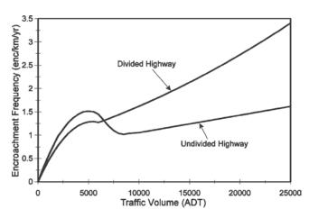
FIGURE 6 Encroachment rates used in Roadside Safety Analysis Program (Mak and Sicking 2003).
