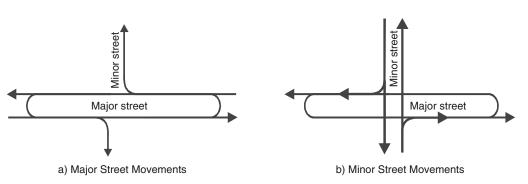
FIGURE 13 MUT left-turn movements (based on Hughes et al. 2010).
