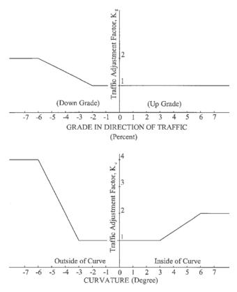
FIGURE 7 Encroachment frequency adjustment factors for curvature (Wright and Robertson 1976).
