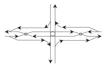
FIGURE 17 Double crossover intersection (Bared et al. 2005).
