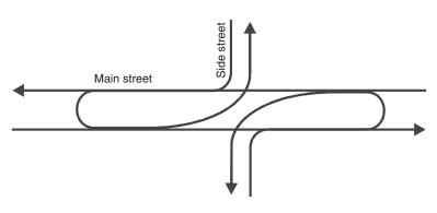
FIGURE 14 Conceptual RCUT configuration with direct left turns from the major road (based on Hughes et al. 2010).
