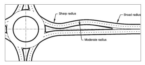
FIGURE 9 Example of approach curvature (Robinson et al. 2000).
