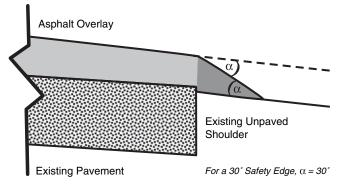
FIGURE 5 Illustration of FHWA's Safety Edge Treatment (Hallmark et al. 2006).
