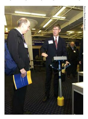
At the 2006 TRB Annual Meeting, Jean-Louis Briaud (*right*) demonstrates the Briaud Compaction Device developed under the NCHRP IDEA program to measure soil modulus at the surface of a compacted layer.
