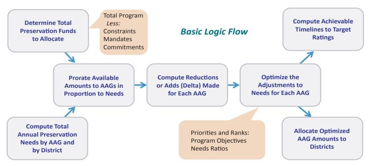
Figure 6-2. Resource allocation model—logic flow.
