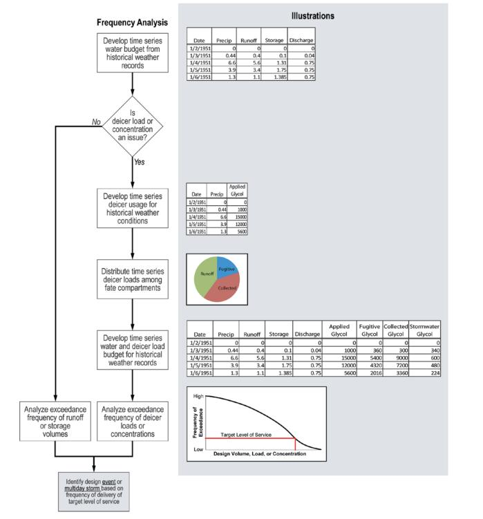
Figure 3-2. Winter design storm frequency analysis process.
