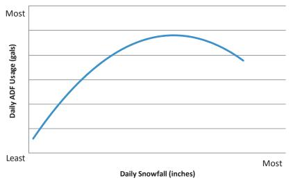
Figure 3-3. Example of how the relationship between daily snowfall and Type I ADF usage can be expressed.
