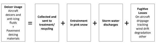
Figure 3-4. Material balance. Adapted from ACRP Report 14 (CH2M HILL et al., 2009).
