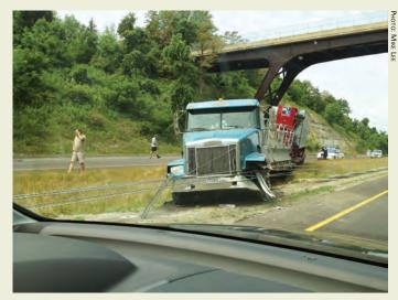
A median cable barrier on I-470 in Ohio prevented this tractor-trailer from reaching the opposite lanes of the highway in a crash. Roadside traversals are among the collision events analyzed by RSAPv3.
