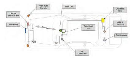
FIGURE 2 DAS schematic view.
