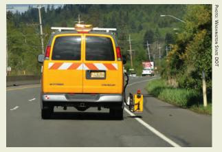
Washington State DOT works with Oregon DOT to rent an expensive, laser-equipped vehicle for collecting road stripe retroreflectivity data. According to the FHWA's Roadway Safety Data Partnership, levels of roadway data practice differ between states; collaborative programs can establish common approaches.
