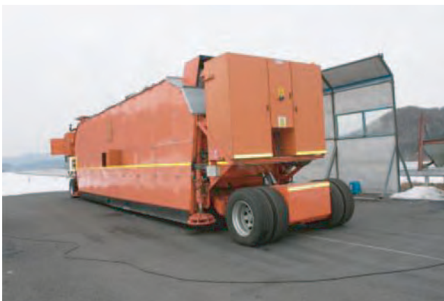
FIGURE 20 China Liaoning Province Communication Research Institute f-sAPT device.
