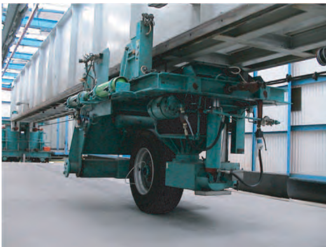
FIGURE 31 LINTRACK f-sAPT device.
