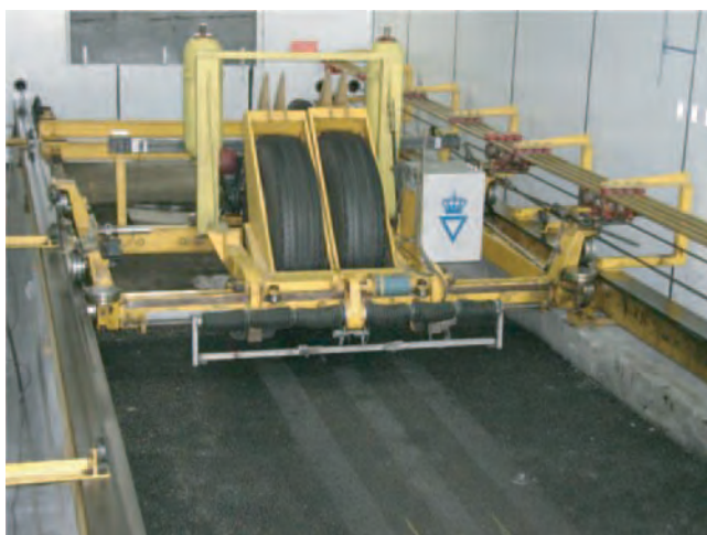
FIGURE 24 Danish road testing machine.
