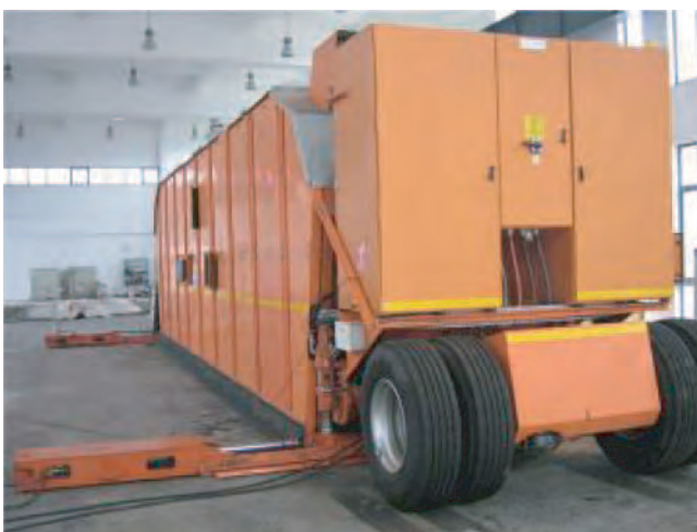
FIGURE 23 Tongji MLS device.
