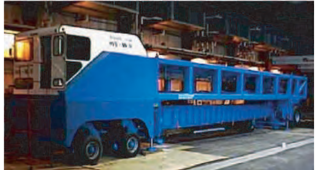
FIGURE 15 USACE CRREL HVS.
