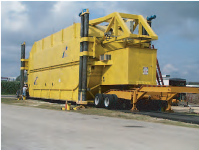
FIGURE 14 Refurbished TxDOT MLS.
