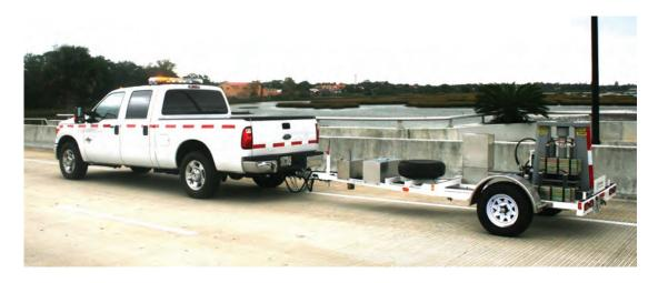
Particular engineers need accurate, complete, and reliable data to manage highway pavements optimally and to diagnose problems efficiently. Drilled core holes and cut trenches historically have yielded pavement samples for analysis. New nondestructive test (NDT) methods, however, can provide greater amounts of data more efficiently and cost-effectively, without damaging pavement or disrupting traffic.
