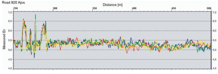
Figure 3.19. Repeatability tests of four GPR runs with 2.2-GHz GSSI system (36).
