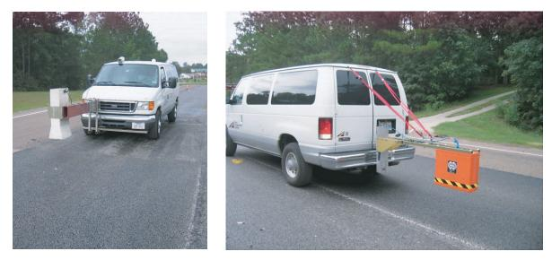
Figure 3.37. 1-GHz (left) and 2-GHz (right) GPR data collection.
