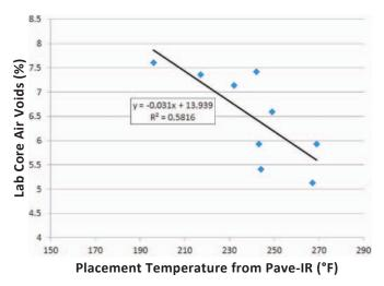
Figure 3.75. Air voids versus placement temperature from Region 1 data.
