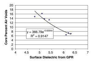
Figure 3.24. Calibration of GPR surface dielectric to core air void content (6).
