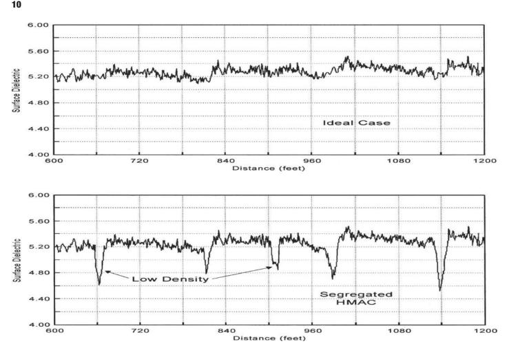
Figure 3.3. Comparison of surface dielectrics measured with GPR of uniform (top) and cyclically segregated (bottom) HMA (2).
