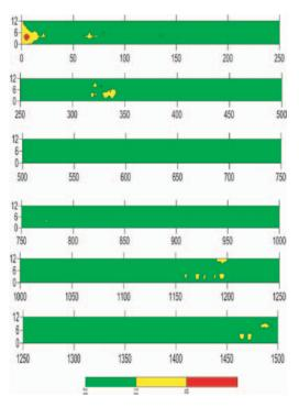
Figure 3.79. Geospatial distribution of air voids on Region 1 project from 1-GHz radar.
