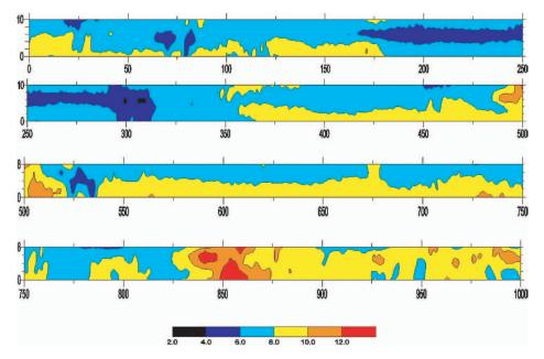
Figure 3.25. In-place percent air voids of new overlay measured with GPR (6).
