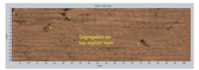
Figure 3.23. Segregation detection with three-dimensional GPR (28). Note that segregation of the larger area is deeper in the asphalt, which can also be seen in the three-dimensional radar GPR time-slice view calculated from a depth of 50 mm. This case presents a 100 m  $\times$  30 m area of an airport runway.
