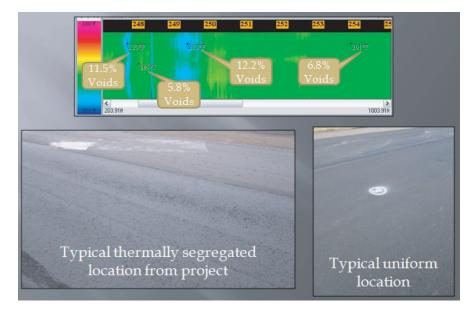
*Figure 3.57. Example of core densities and mat appearance with thermal segregation from demonstration in Region 3.*
