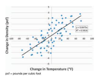
*Figure 3.76. Density differentials versus temperature differentials from Region 1 demonstration.*
