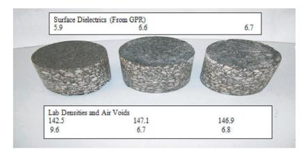
Figure E.2. Comparing field dielectrics with laboratory-measured properties.
