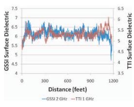
Figure 3.44. Surface dielectrics measured with 1-GHz and 2-GHz systems on Region 4 demonstration project.
