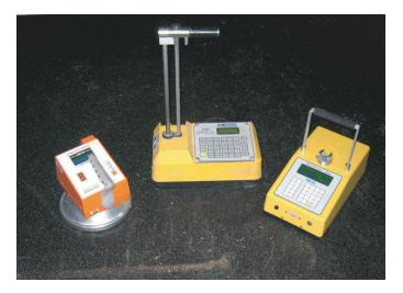
*Figure 3.26. PQI, nuclear density gauge, and Pavetracker Plus.*
