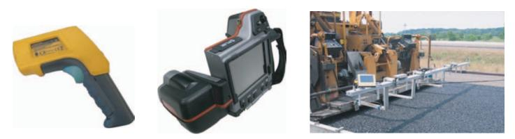
Figure 3.4. Spot radiometer, IR camera, and IR bar measurement systems.
