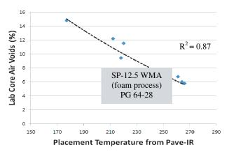
Figure 3.58. Air voids versus placement temperature from Region 3 project.
