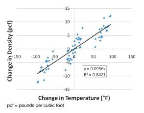
*Figure 3.49. Density differentials versus temperature differentials from Region 2 data.*
