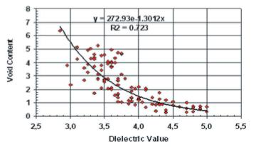
Figure 3.20. Relationship between HMA void content and dielectric values (31). Note that dielectric values are measured with capacitance-based Percometer surface probe.
