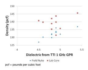
Figure 3.42. Lack of correlation between GPR and laboratory density with Region 4 data.
