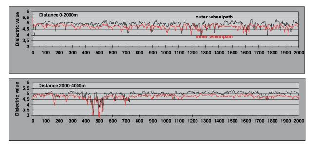
Figure 3.21. Dielectric value of asphalt at Ylinampa (17).
