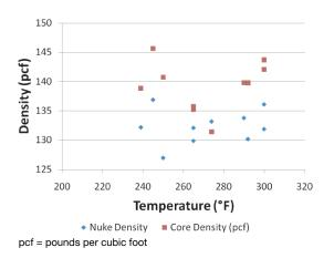
Figure 3.40. Lack of correlation between temperature and density with Region 4 data.
