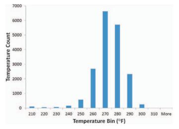
Figure 3.10. Histogram of measured mat placement temperatures from modified paving operation (9).
