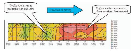
Figure 3.11. Surface temperature profile from the University of Twente (10).
