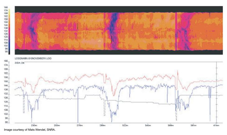
Figure 3.12. Thermal profile output from line scanner system in Sweden.
