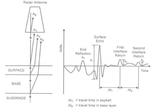
Figure 3.16. Example signal from a GPR pulse (12).
