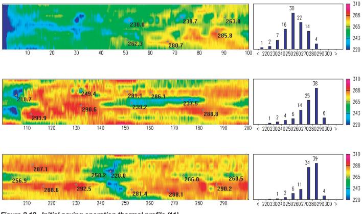
Figure 3.13. Initial paving operation thermal profile (11).
