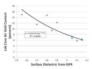
Figure 3.63. Calibrating GPR to predict in-place air voids from Region 3 data.
