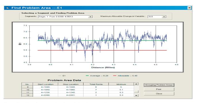
Figure E.1. Plot of computed surface dielectric versus distance along the project.
