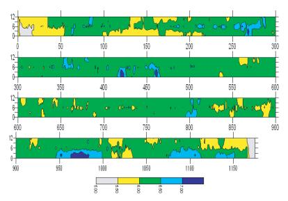
Figure 3.39. Surface dielectric measured with 2-GHz GPR system on Region 4 demonstration.
