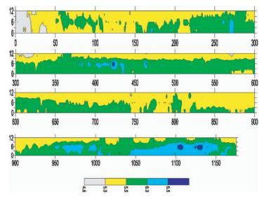
Figure 3.38. Surface dielectric measured with 1-GHz GPR system on Region 4 demonstration.
