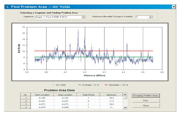
Figure E.4. Plot of computed air voids for a single GPR run.
