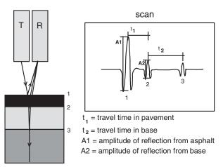
Figure C.1. Operational principle of horn antenna.
