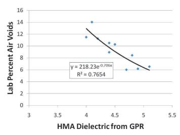
Figure 3.50. Calibrating GPR to predict in-place air voids from Region 2 data.
