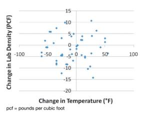
Figure 3.41. Lack of correlation between temperature and density differentials with Region 4 data.
