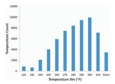
Figure 3.9. Histogram of measured mat placement temperatures from initial paving operation (9).
