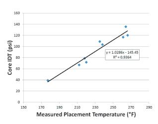
Figure 3.62. Core IDT versus measured placement temperature from Region 3.
