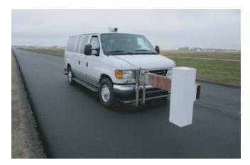
Figure 3.56. GPR data collection on Region 3 demonstration project.
