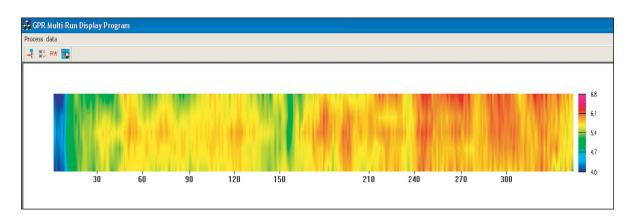
Figure E.5. Surface dielectric plot from five parallel GPR runs.
