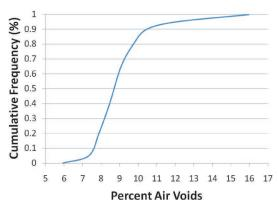
Figure 3.52. Expected air void distribution for SP-12.5 HMA in Region 2.
