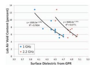
Figure 3.77. Calibrating GPR to predict in-place air voids for Region 1 demonstration.
