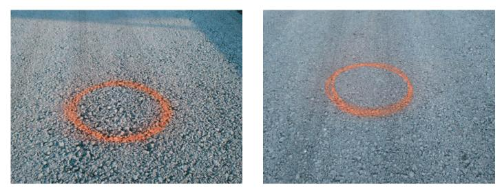
Figure 3.14. Thermal cold spot (left) and normal (right) locations on HMA mat (11).
