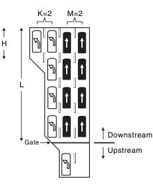
Figure 2.13. Illustration of a link with dual left turn pockets.
