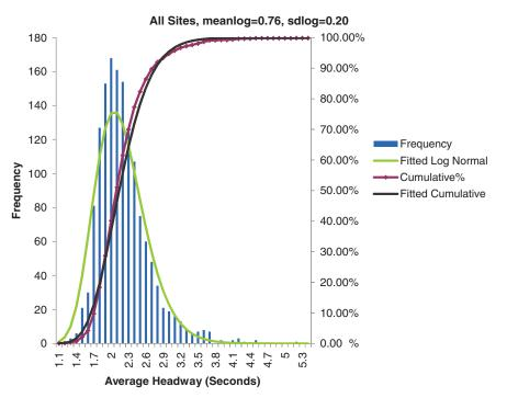
Figure ES.2. Stochastic headway/capacity flow distribution for arterials.
