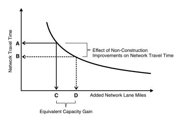
Figure 4.8. Equivalent capacity gain concept.
