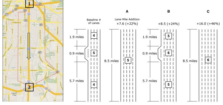
Figure 4.9. Illustrations of three physical lane addition scenarios.
