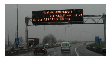
Figure 3.3. VMS queue-based routing in the Netherlands.
