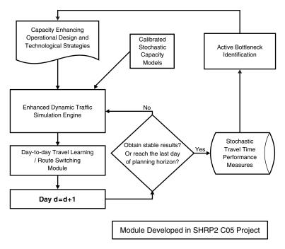
Figure ES.4. Module developed in SHRP 2 C05 project as a capacity-enhancing strategy evaluation framework.
