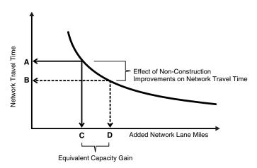
Figure 1.1. Equivalent capacity gain concept.
