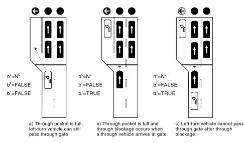
Figure 2.15. Illustration of through blockage events.
