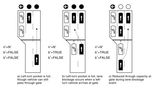
Figure 2.14. Illustration of left turn pocket blockage events.
