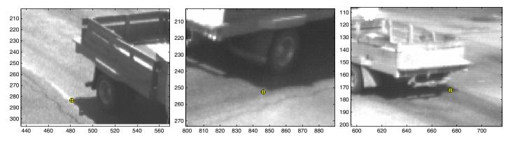
Figure 7.12. Simultaneous images (zoomed in) from the NE, SE, and SW cameras. The marked point is coincident in time and in 3-D world coordinates. Scales are pixel coordinates.
