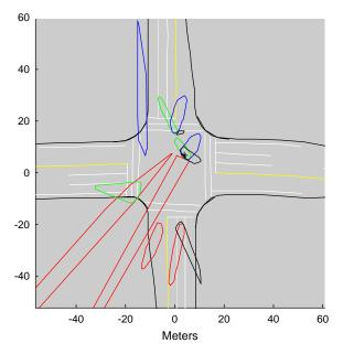
Figure 9.5. Multicamera blob projections at time t<sub>ref</sub>. The black star shows the location of the centroid of associated clusters. Colors denote camera source: NE, blue; SE, red; SW, green; and NW, black.
