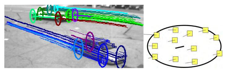
Figure 8.3. The clustering algorithm uses corner feature grouping and is sensitive to distances in the image. Left: Feature tracks and clusters on two vehicles (parking lot test at UMTRI). Right: Dispersion and mean velocities are recorded as part of the cluster properties.
