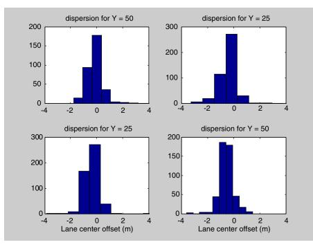
Figure 11.5. Frequency distributions for lateral dispersion within the lane for through vehicles. North-to-south movement: upper left, 50 m north; upper right, 25 m north; lower left, 25 m south; and lower right, 50 m south.
