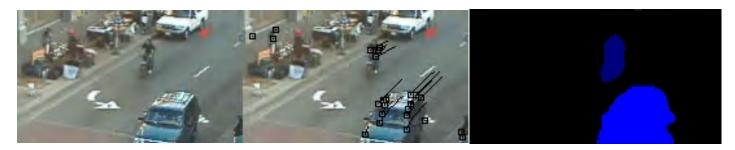
Figure 8.2. An example video image (left), a corner feature detection and tracking result (center), and a background subtraction result (right).
