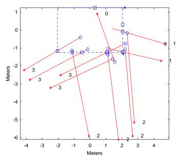
Figure 9.8. Cluster localization using a vehicle rectangle (vehicle coordinate system:  $X_v$  is horizontal,  $Y_v$  is vertical; units are in meters). Numeric values adjacent to cluster lines indicate the camera location: 0 = NE, 1 = SE, 2 = SW, and 3 = NW.
