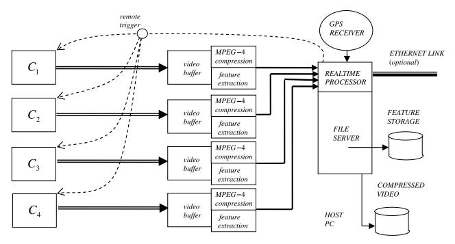
Figure 6.5. Camera, data acquisition and preprocessing system (CDAPS).
