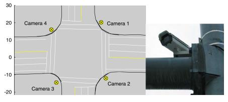
Figure 7.8. Camera positions. Left: Plan view. Right: Mounting positions are on traffic signal mast arms, close to the signal mast (Camera 3 is shown here).
