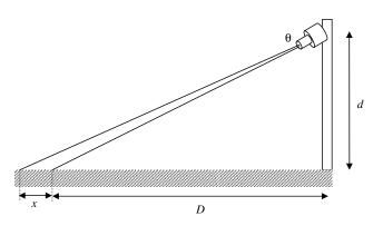
Figure 6.1. Basic camera geometry and resulting pixelation error.
