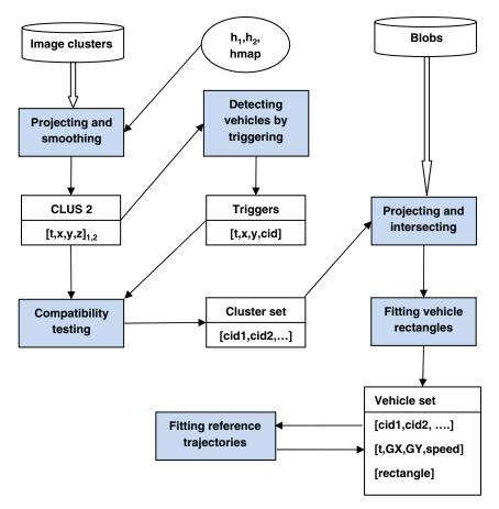
Figure 9.13. Block diagram summary of basic vehicle trajectory estimation.
