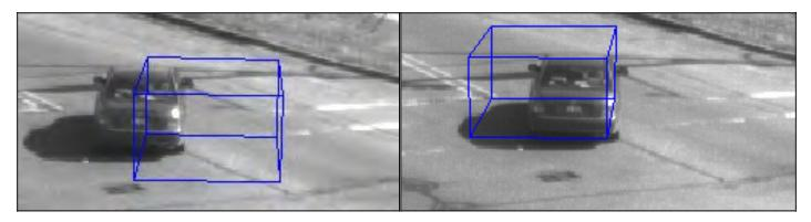
Figure 10.4. Lateral offset attributable to vehicle shadow. No shadow compensation has been applied in this analysis. Time:  $t_{ref} + 1$ .
