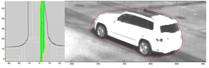
Figure 8.6. World view and camera view of cluster tracks on a single vehicle (through vehicle traveling north).
