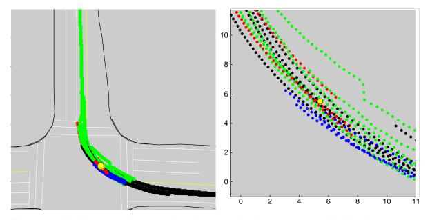
Figure 9.4. Multicamera cluster tracks using a nominal 0.5-m assumed height above ground. Left plot shows detail. Yellow dot is reference track at reference time. Tracks are seen from cameras at the NE (blue), SE (red), SW (green), and NW (black) corners. Scales are in meters.
