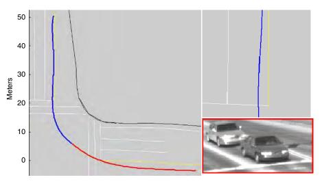
Figure 9.11. Basic vehicle fitted path (red: using outgoing cluster; blue: using incoming cluster). The right plot shows a detail of the track near the stop bar; corresponding vehicle image is for the front car at the stop bar.
