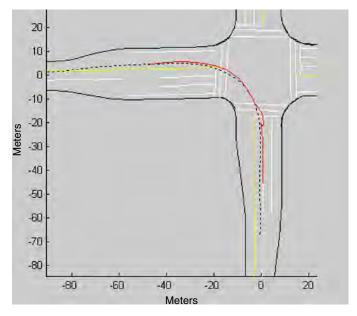
Figure 10.5. Kalman filter estimation of vehicle path.
