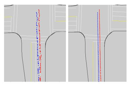
Figure 9.1. A single-cluster track resolved in world coordinates at an assumed height of 0.5 m (blue) and 1.5 m (red), with vehicle traveling to the north, viewed from NE camera.
