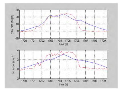
Figure 11.11. LTAP/OD conflict—yaw rate and lateral acceleration estimates for the turning vehicle. Blue: video based; red dashes: vehicle based.
