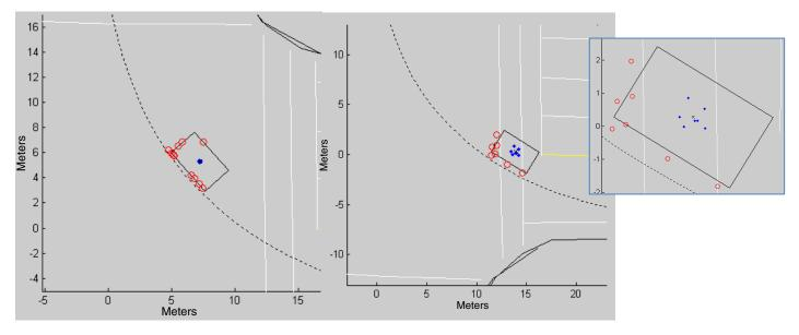
Figure 10.2. Example of position refinement. Red circles are cluster projections; blue dots are centroid estimates. Left: At reference time. Right: At time  $t_{ref} + 1$ . Zoomed image also is at time  $t_{ref} + 1$ .
