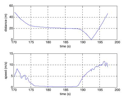
Figure 9.12. Speed and distance estimates from basic track fitting.
