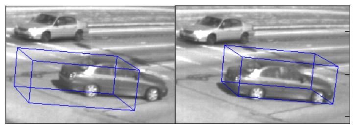
Figure 10.3. Effect of position refinement. Left: Initial approximation from single cluster and nominal height estimate. Right: Uses position refinement by coordinate offsets. Time:  $t_{ref}$  + 0.7.
