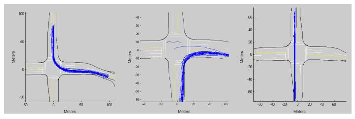
Figure 11.4. Samples of detected trajectories in selected directions. The central plot shows a single corrupted trajectory. Less than 1% of trajectories are this type and can be removed by screening.
