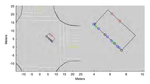
*Figure 9.9. Fitted rectangle and associated cluster points, including close-up (right plot). Colors according to camera corner location: NE, red; SE, green; SW, blue; and NW, black.*
