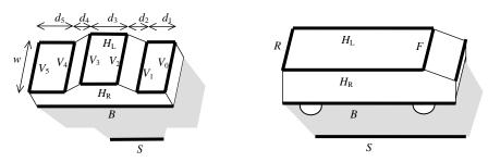
Figure 3.3. The wireframe models used by the NGSIM system to detect a passenger vehicle (left) and a container truck (right).
