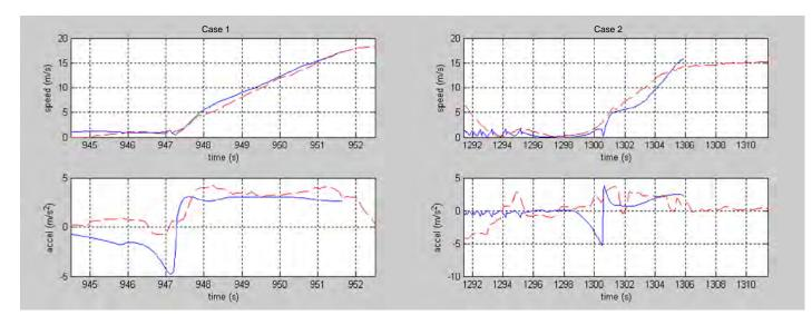
Figure 11.8. Speed and acceleration estimates for slow-turning vehicles, right turn into path. Blue: video measurement; red dashes: vehicle measurement.
