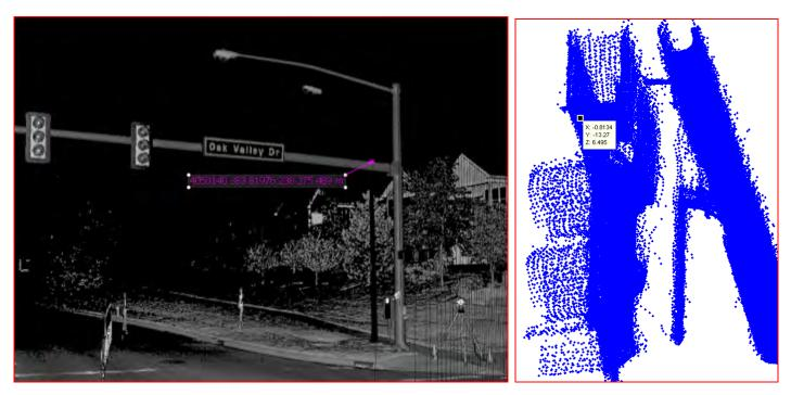
Figure 7.5. Virtual view from lidar survey using Leica TruView software. Right: detail of reference point on traffic signal used for camera calibration.
