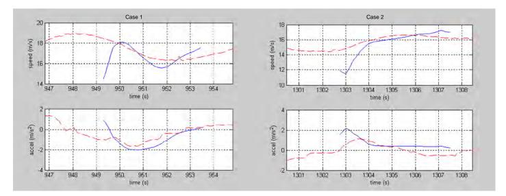
Figure 11.7. Speed and acceleration estimates for through vehicles, right turn into path. Blue: video measurement; red dashes: vehicle measurement.
