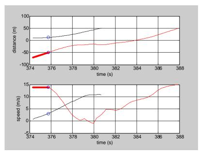
Figure 12.5. RTIP conflict. Red: through vehicle; black: turning vehicle; blue circle: point of minimum time to collision.
