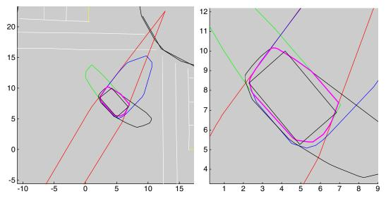
Figure 9.6. Detail and vehicle localization by intersecting blobs. Blob color codes are the same as in Figure 9.5, with the addition of a magenta bounding polygon and fitted rectangle (black). Distances are in meters.
