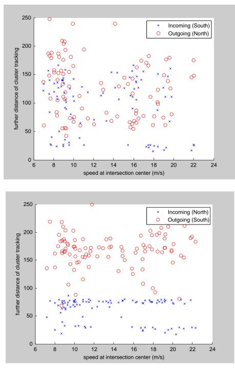
Figure 11.3. Lengths of cluster tracks: through vehicles, north and south directions.
