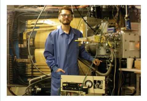
FIGURE FEL 1 Graduate student Paul Ellison with the Berkeley Gas-Filled Separator, used for studying the chemistry and physics of the heaviest elements. SOURCE: Image courtesy of PT Lake.
