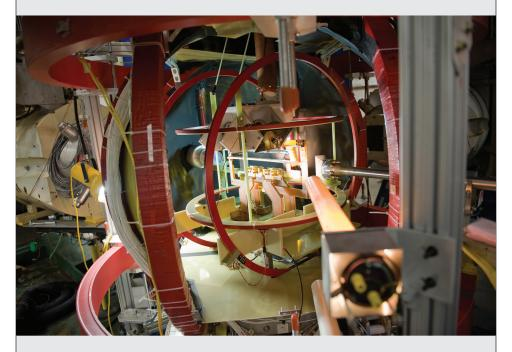
FIGURE 2.5.1 Photograph of JLAB's polarized helium-3 target, used to make precision electron scattering measurements of the charge, magnetism, and spin distributions of the neutron. SOURCE: Courtesy of JLAB.
