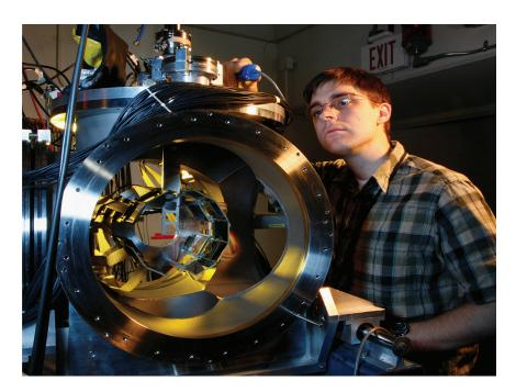
FIGURE FEL 4 Patrick O'Malley uses the ORNL accelerator and the ORRUBA array of positionsensitive silicon strip detectors to study nuclear reactions that help us understand how the elements are synthesized in stars. SOURCE: Patrick O'Malley.
